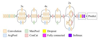
Fig. 6. Convolutional Neural Network Architecture Inception v3
