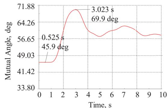
Fig. 5. Plot of the mutual angle ( $\delta$ ) between the «Ekibastuz» substation and «Almaty» substation based on simulation results in PowerFactory DigSILENT
