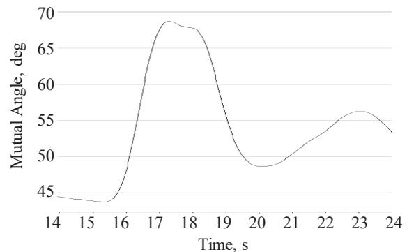
Fig. 4. Plot of the mutual angle ( $\delta$ ) between the «Ekibastuz» substation and «Almaty» substation according to data from the Wide Area Measurements System
