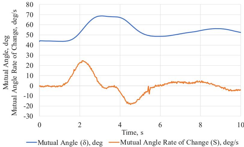
Fig. 3. Plots of the mutual angle ( $\delta$ , deg) and its Rate of Change ( $S$ , deg/s) between the «Ekibastuz» substation and «Almaty» substation at the power surge from the Central Asia Unified Energy System in the amount of about 700 MW
