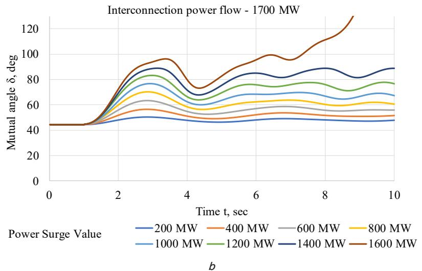
Fig. 6. Plots of the mutual angle ( $\delta$ ) at power surges of different magnitudes and at different loads of the «North-South» interconnection: *a* – power flow of 2,100 MW; *b* – power flow of 1,700 MW
