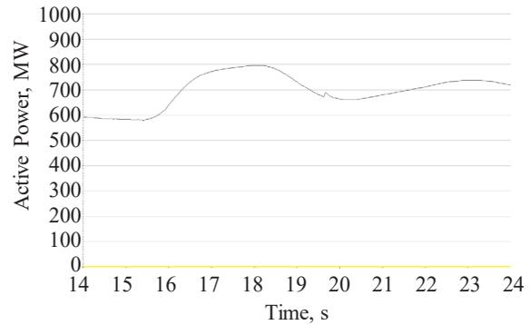
Fig. 2. Plot of change in the active power flow along the «North-South» interconnection from the Wide Area Measurements System with a power surge from the Central Asia Unified Energy System of about 700 MW
