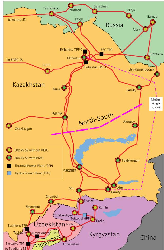
Fig. 1. Schematic map of 500 kV power grids of the Republic of Kazakhstan Unified Energy System included in the «North-South» interconnection
