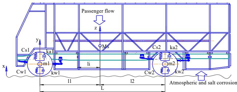
Fig. 1. Scheme for assessing the durability of the bus body on the frame chassis
