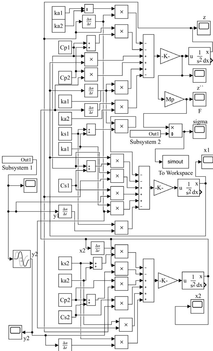
Fig. 3. Simulation model in Matlab Simulink, based on the developed approach to assessing the durability of A bus body on the frame chassis
