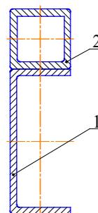
Fig. 2. The studied cross-section of the bus body on the frame chassis: 1 – frame; 2 – body frame element
