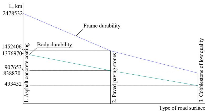
Fig. 5. Dependences of durability of the body frame and frame of the bus «Etalon» BAZ-A079 on the type of road surface
