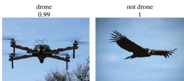
Fig. 6. Example of testing a trained neural network for object classification
