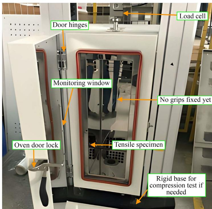
Fig. 1. Thermal tensile test device [15]
