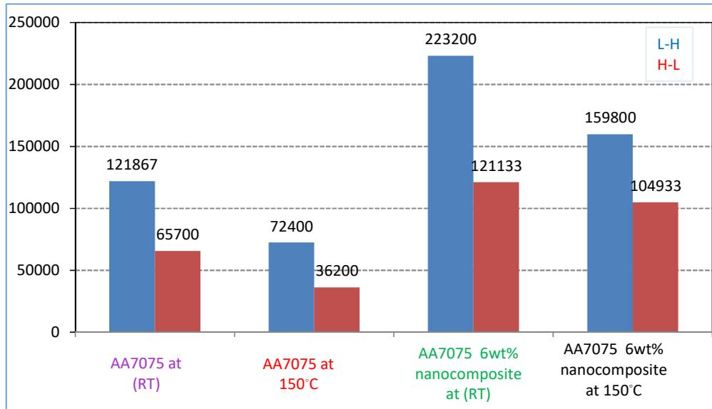
Fig. 4. Variable fatigue loading fatigue result at (RT) and (150 °C)
