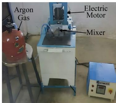
Fig. 2. Manufacturing process of nanocomposite materials [10]
