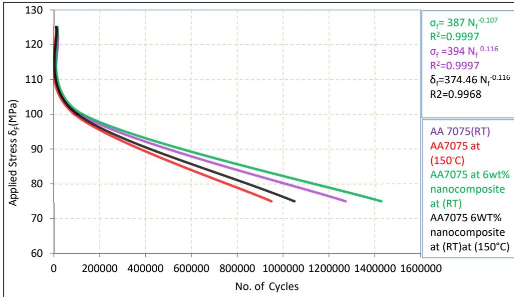
Fig. 3. Constant S-N curve at four cases of testing
