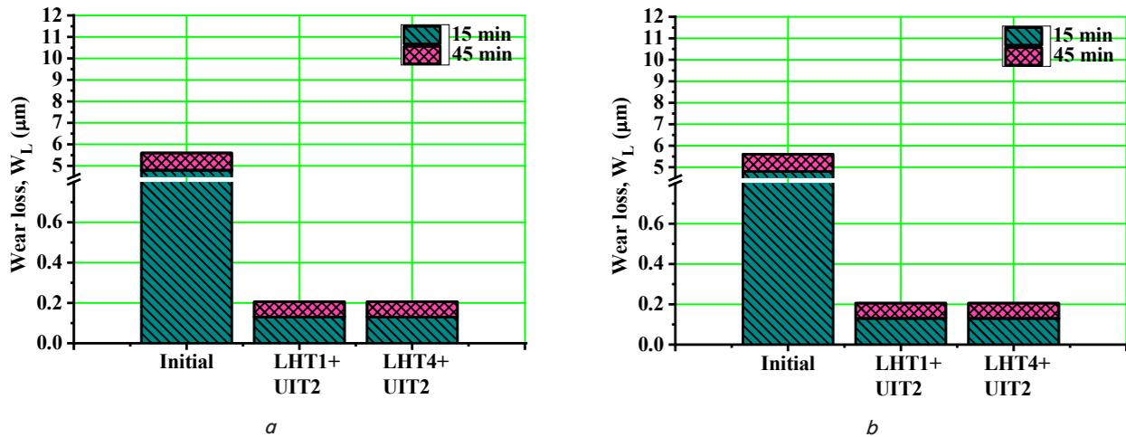
Fig. 4. Wear loss values under dynamic load: *a* – AISI 1045 steel; *b* – AISI D2 steel
