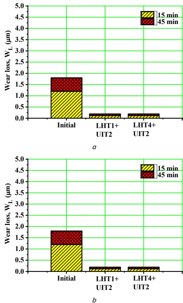
Fig. 3. Wear loss values under quasi-static load: a – AISI 1045 steel; b – AISI D2 steel
