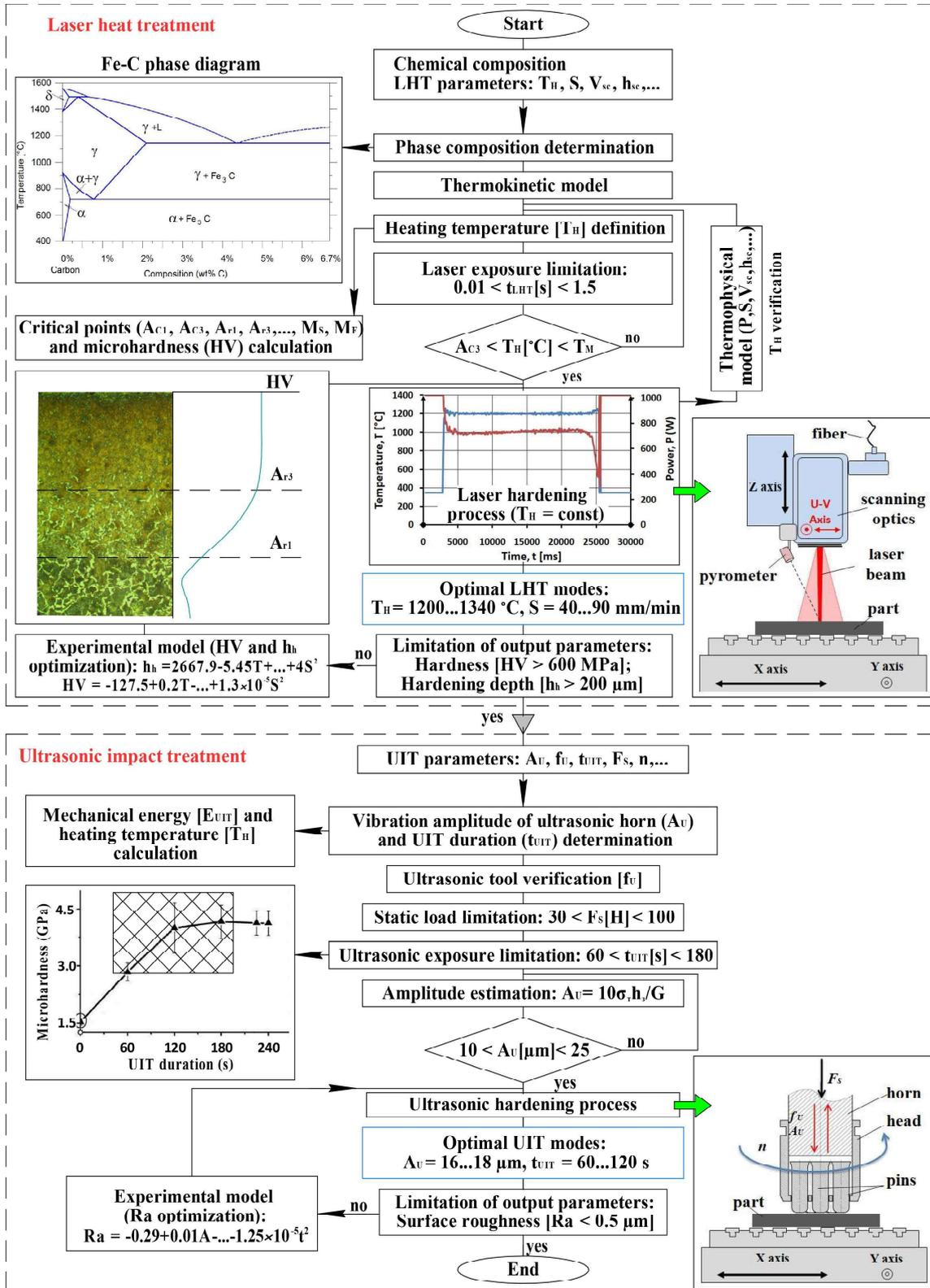
Fig. 5. Determination algorithm of technological parameters of combined laser-ultrasonic treatment of structural and tool steels
