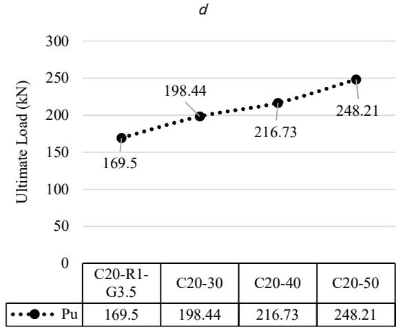
Fig. 4. Analytical results regarding the cracking and ultimate loads: *a* – cracking loads of concrete corbels; *b* – ultimate loads of concrete corbels; *c* – cracking loads of concrete corbels; *d* – ultimate loads of concrete corbels; *e* – cracking loads of concrete corbels; *f* – ultimate loads of concrete corbels
