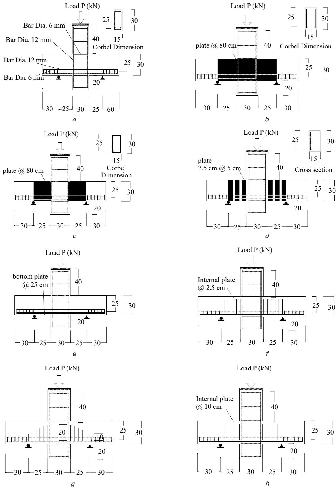
Fig. 3. Geometrical details of reinforced corbels: *a* – C20-R1-G3.5; *b* – ECP-800; *c* – ECP-S500; *d* – ECP-P250; *e* – ECP-UP550; *f* – ICPRS & ICP-250; *g* – ICP-V50; *h* – ICP-125
