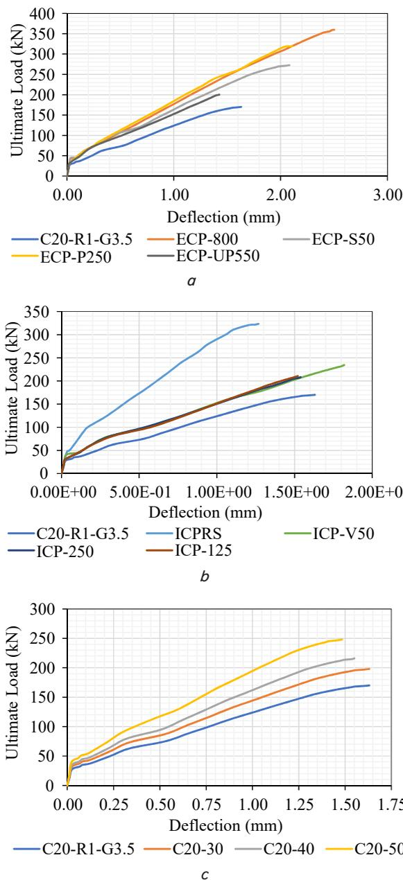
Fig. 5. Analytical results regarding the cracking and ultimate loads showing the maximum displacement of concrete corbels: *a* – external strengthened specimens; *b* – internal strengthened specimens; *c* – strengthened specimens with compressive strength
