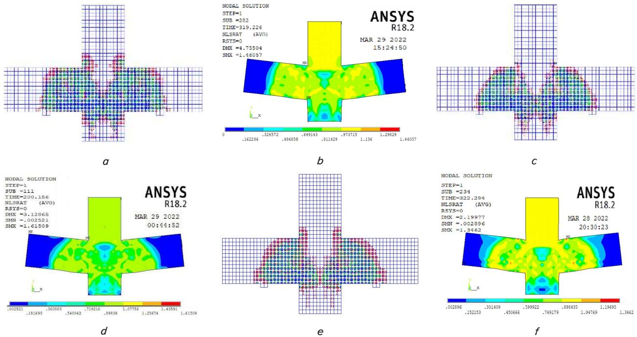
Fig. 7. Analytical results regarding the crack pattern and stress distribution: *a* – crack pattern and stress distribution of ECP-P250 model; *b* – crack pattern and stress distribution of ECP-P250 model; *c* – crack pattern and stress distribution of ECP-UP550 model; *d* – crack pattern and stress distribution of ECP-UP550 model; *e* – crack pattern and stress distribution of ICPRS model; *f* – crack pattern and stress distribution of ICPRS model
