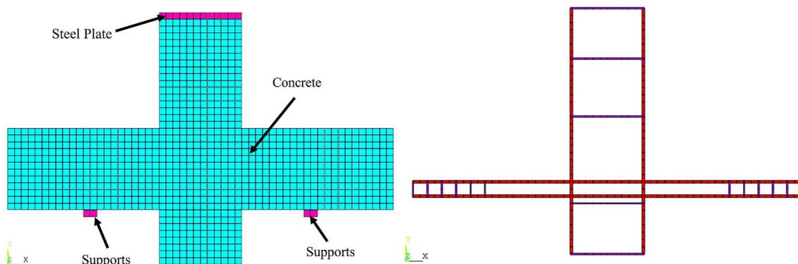
Fig. 1. The model of the RC corbels: a – finite element model shows the mesh of concrete; b – glass fibers reinforced polymers rebar in ANSYS
