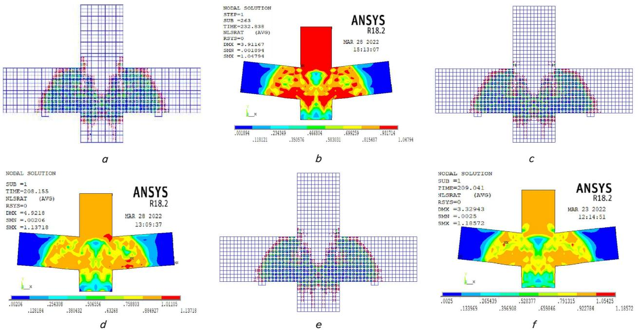
Fig. 8. Analytical results regarding the crack pattern and stress distribution: *a* – crack pattern and stress distribution of ICP-V50 model, *b* – crack pattern and stress distribution of ICP-V50 model; *c* – crack pattern and stress distribution of ICP-250 model; *d* – crack pattern and stress distribution of ICP-250 model; *e* – crack pattern and stress distribution of ICP-125 model; *f* – crack pattern and stress distribution of ICP-125 model
