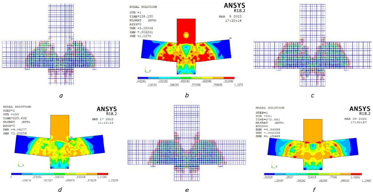
Fig. 6. Analytical results regarding the crack pattern and stress distribution: a – crack pattern and stress distribution of C20-R1-G3.5 model; b – crack pattern and stress distribution of C20-R1-G3.5 model; c – crack pattern and stress distribution of ECP-800 model; d – crack pattern and stress distribution of ECP-800 model; e – crack pattern and stress distribution of ECP-S500 model; f – crack pattern and stress distribution of ECP-S500 model
