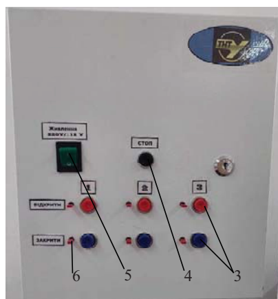
Fig. 13. Control panel: 1 – DC power supply unit 220/12V (5A); 2 – control relay of actuators; 3 – buttons "Open", "Close"; 4 – "Stop" button; 5 – power switch 220V; 6 – fuse (220V); 7 – Wi-Fi controller; 8 – LED indicators; 9 – 12V power off button when opening the control cabinet
