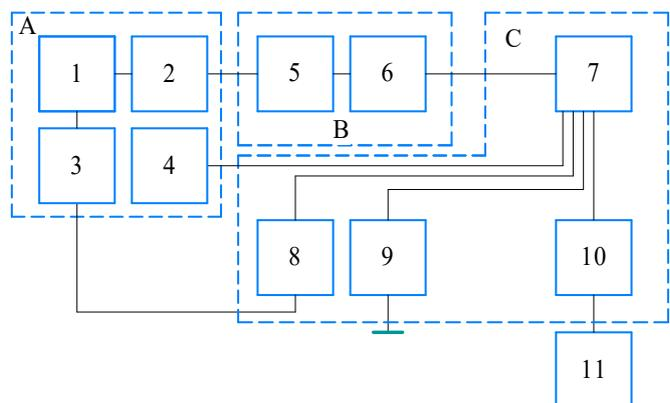
Fig. 2. Block diagram of an installation for obtaining an underwater electrical explosion: A – remote control; B – HPT; C – energy storage with protection system; 1 – power supply 220 V; 2 – current limiting element; 3 – emergency shutdown system; 4 – high voltage indicator; 5 – transformer; 6 – high voltage rectifier; 7 – energy storage unit; 8 – protection system; 9 – residual stress relief system; 10 – air gap; 11 – working part for crushing and grinding quartz mineral
