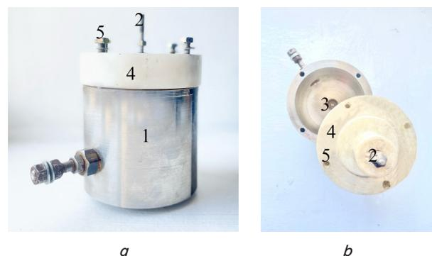
Fig. 3. The working part of the experimental plant for crushing and grinding quartz mineral: a – main body; b – working electrodes; 1 – cylindrical housing with a diameter of 100 mm; 2 – positive electrode with a diameter of 3 mm; 3 – negative electrode; 4 – caprolon cap with a diameter of 110 mm; 5 – fasteners
