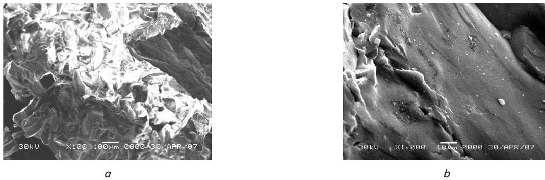
Fig. 6. Electronic images of powdered quartzite after electrohydroimpulse treatment with expansion: *a* – with a magnification of 100 times; *b* – with a magnification of 1,000
