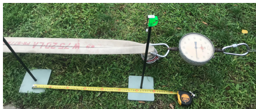
Fig. 5. Conducting a full-scale experiment using latex pressure fire hoses with a length of 1960 cm and diameter D=77 mm: a – schematic; b – fragment of the experiment
