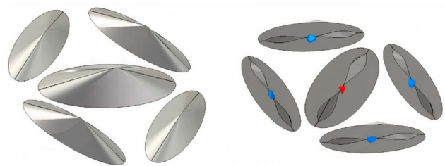
Fig. 3. Ultra-wideband radar, where the central antenna is the emitter; antennas at the edges – receivers with different polarization [18]
