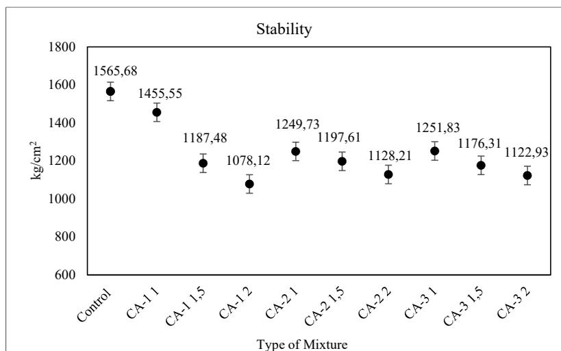
Fig. 3. Marshall stability test results
