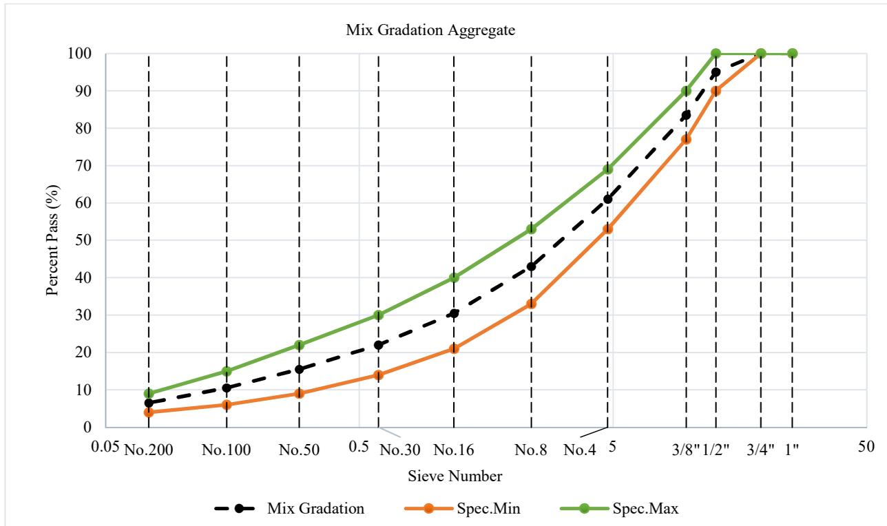
Fig. 1. Combined Aggregate Gradation
