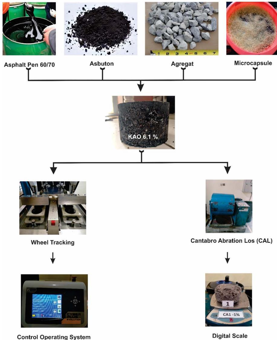
Fig. 2. Experiment testing set up
