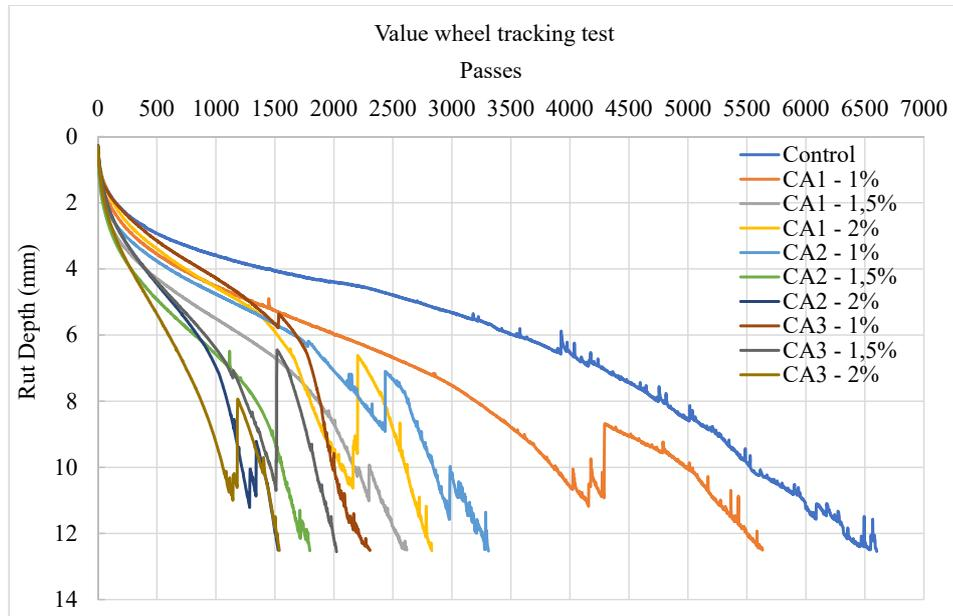
Fig. 4. Wheel Tracking Test Result
