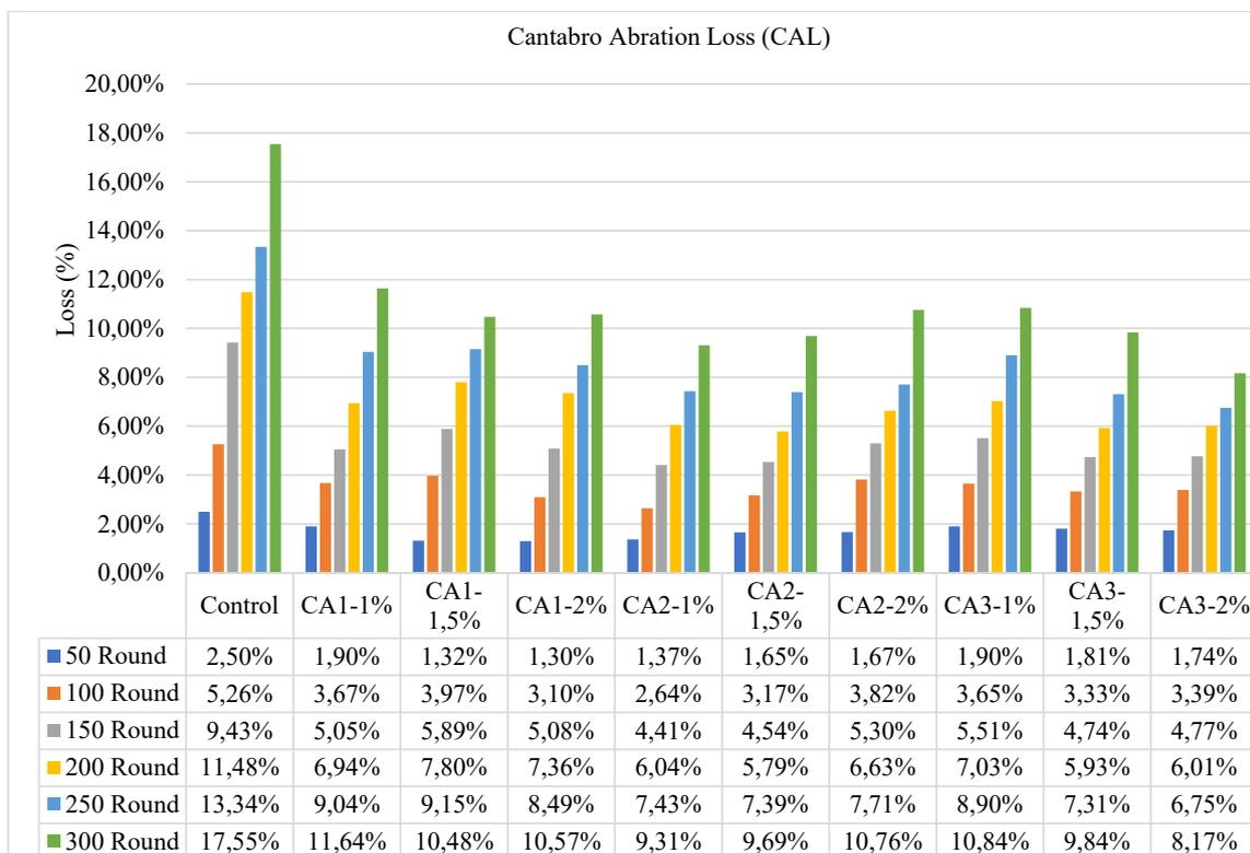
Fig. 5. Graph of Cantabro Abrasion Loss (CAL) test results
