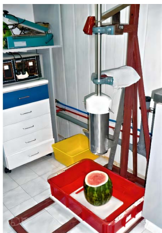
Fig. 3. Watermelon pulp extraction device
