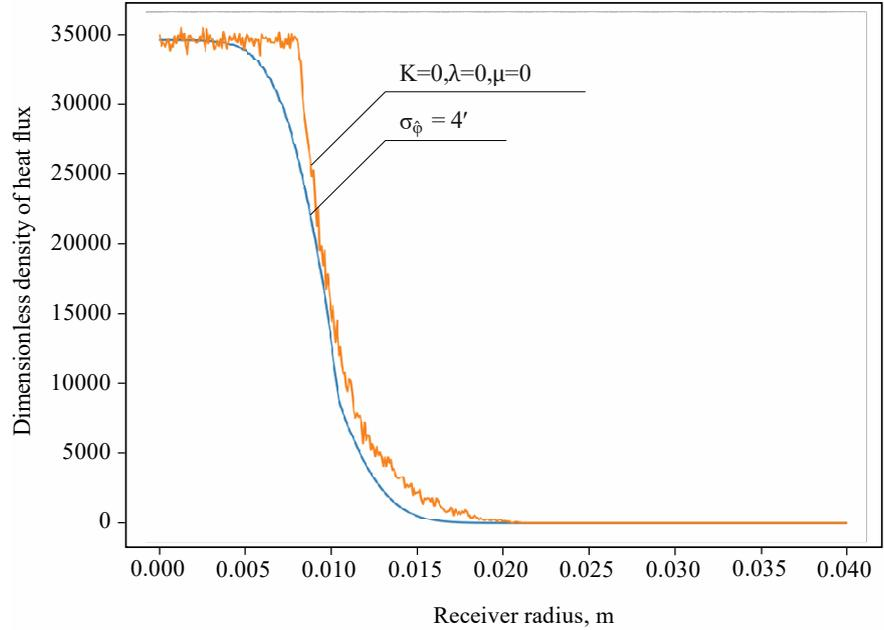
Fig. 4. Comparison of heat flux density distribution obtained by analytical ( $\sigma_{\varphi} = 4'$ ) and numerical methods (ideal concentrator)
