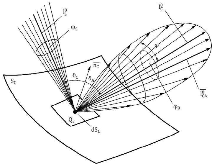
Fig. 1. Scheme of reflection of solar radiation from the surface of the concentrator
