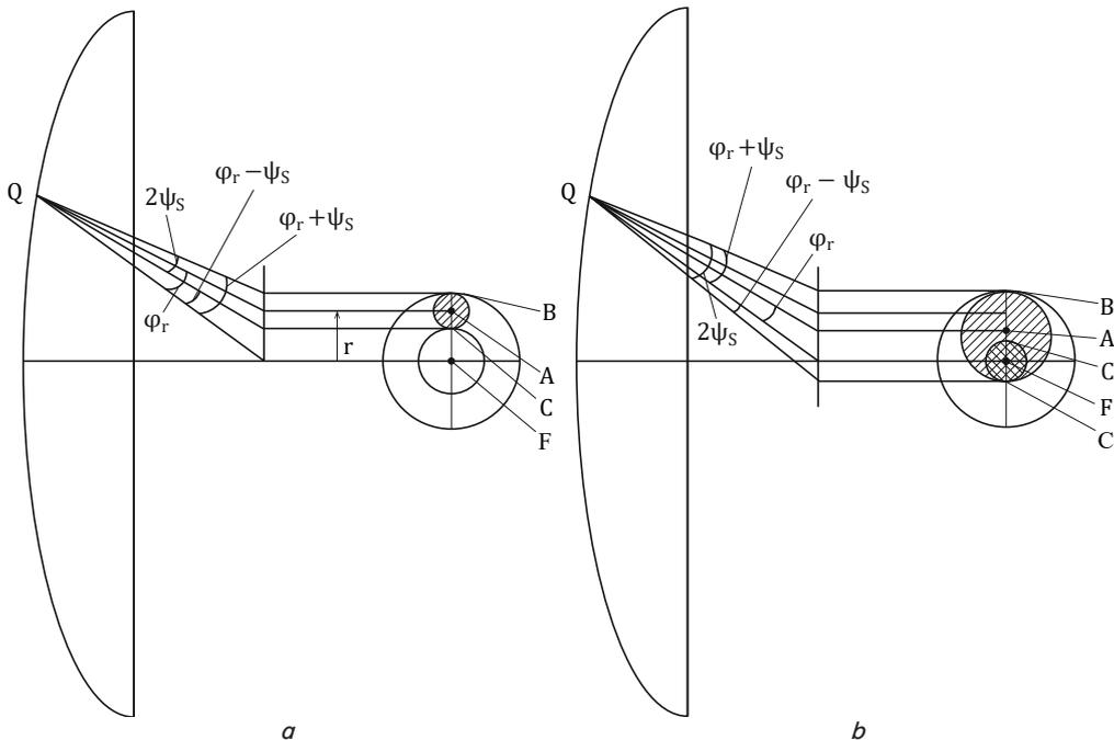
Fig. 3. Irradiation of a point in the focal plane by the annular zone of the concentrator:  $a - \varphi_r \geq \psi_s$ ;  $b - \varphi_r \leq \psi_s$
