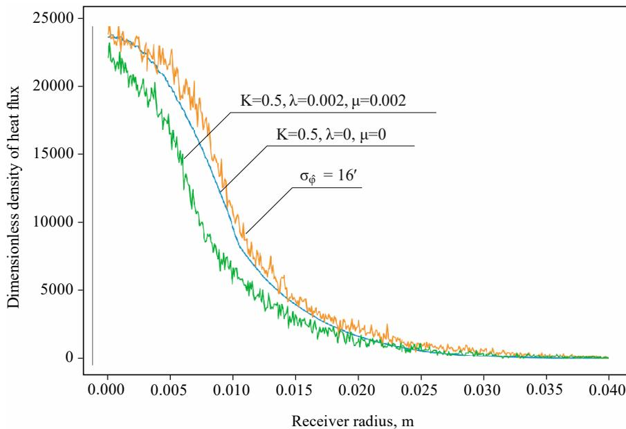
Fig. 5. Comparison of heat flux density distributions obtained by the analytical method ( $\sigma_{\varphi} = 16'$ ) and the numerical method (real concentrator)
