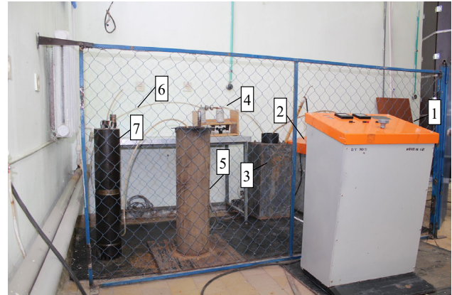
Fig. 2. The appearance of an electrohydraulic installation and an electrohydraulic drill
