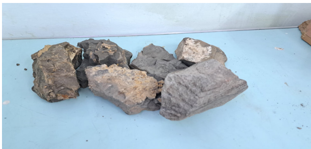
Fig. 1. Photos of stones before processing (53÷78 mm)
