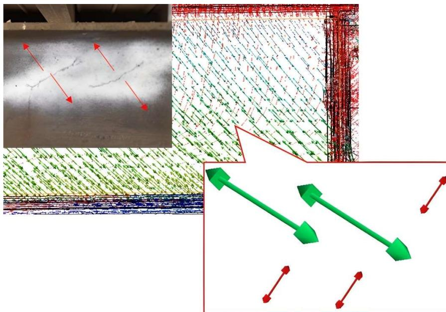
Fig. 15. The direction of the principal stresses under calculation mode IV and the actually detected defects of the girder beam
