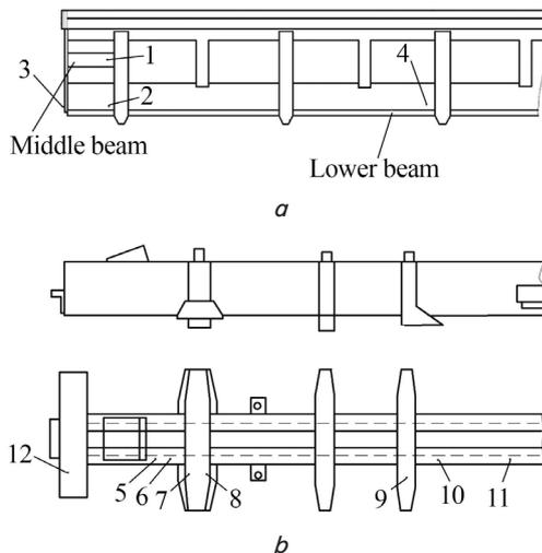
Fig. 1. The diagram of the installation of strain gauges on the load-bearing structures of the dump car: a – the upper frame and the side wall of the car; b – the girder beam of the car
