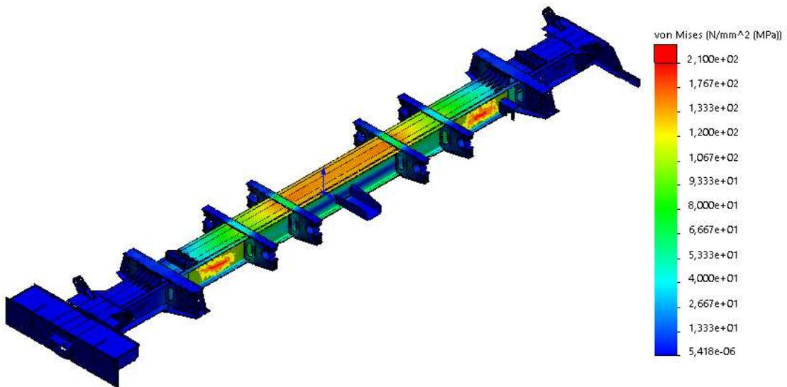
Fig. 14. The diagram of the equivalent stresses of the girder beam of the lower frame of the dump car, model 31-638, according to mode IV
