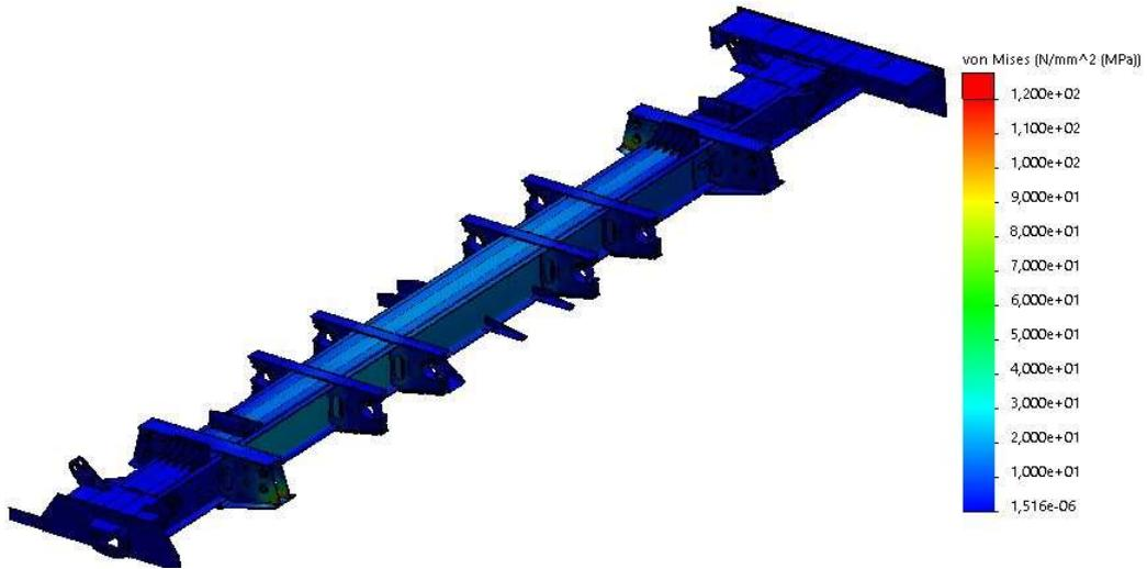
Fig. 8. The diagram of the equivalent stresses of the girder beam of the lower frame of the dump car, model 31-638, according to mode  $II_{rm1}$
