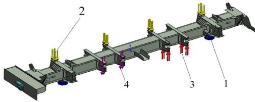
Fig. 13. Calculation diagram of the loading of the girder beam of the lower frame of the dump car, model 31-638, (mode IV): 1 – resting the body on the bogie; 2 – cargo mass and evenly distributed mass of body elements at the beginning of unloading; 3 – unloading forces acting on the elements of the lower frame from the working cylinder; 4 – reactions acting on the elements of the lower frame from the jammed cylinder
