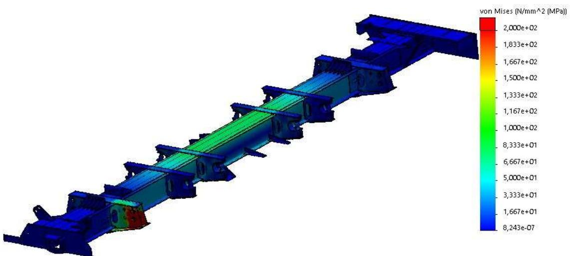
Fig. 10. The diagram of the equivalent stresses of the girder beam of the lower frame of the dump car, model 31-638, according to mode  $II_{rm3}$
