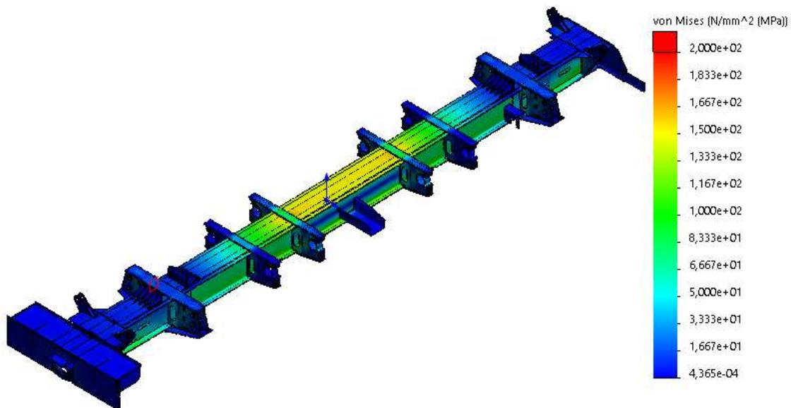
Fig. 12. The diagram of the equivalent stresses of the girder beam of the lower frame of the dump car, model 31-638, according to mode III<sub>e</sub>
