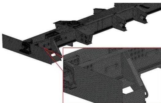
Fig. 3. Finite element model of the girder beam of the lower frame of the dump of car model 31-638
