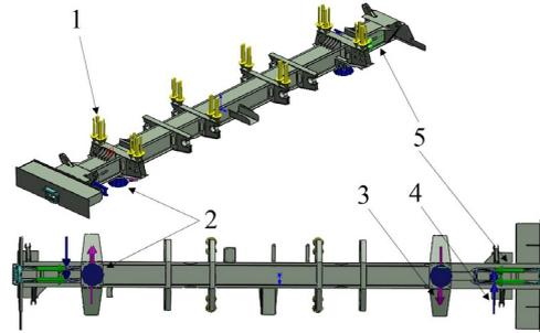
Fig. 4. Calculation scheme of the lower frame of the dump car: 1 – mass of cargo and evenly distributed mass of body elements; 2 – leaning the body on the bogie; 3, 4 – lateral forces; 5 – compression forces from the automatic coupling
