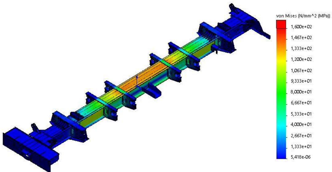
Fig. 7. The diagram of the equivalent stresses of the girder beam of the lower frame of the dump car, model 31-638, according to mode II<sub>odc</sub>
