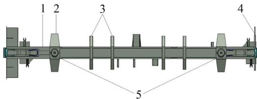
Fig. 2. Spatial model of the lower frame of the dump car (bottom view): 1 – spinal beam; 2 – pivot beam; 3 – cylindrical beam; 4 – end beam; 5 – pivot unit
