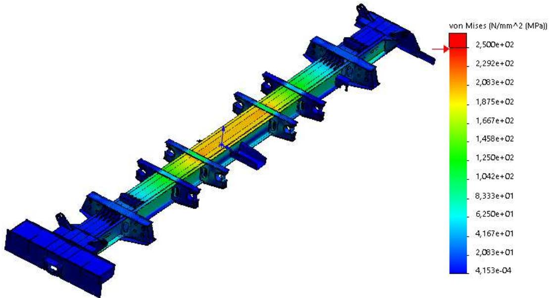
Fig. 11. The diagram of the equivalent stresses of the girder beam of the lower frame of the dump car, model 31-638, according to mode III<sub>c</sub>
