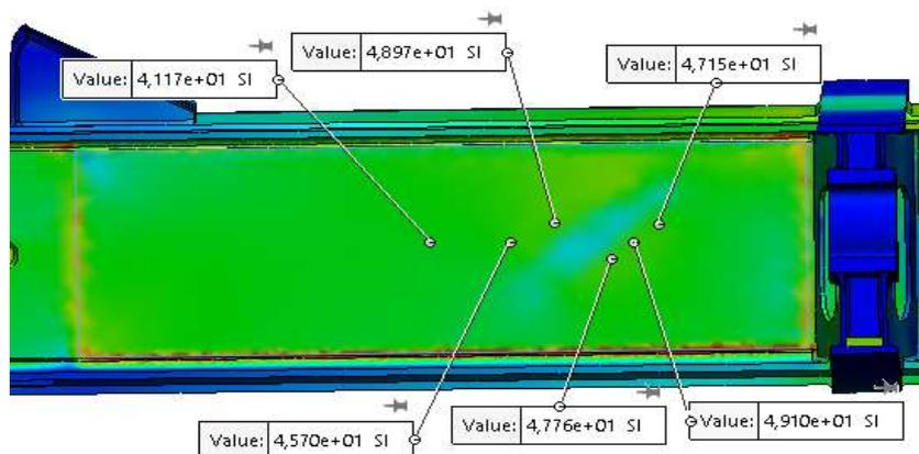
Fig. 16. Diagram of maximum tangential stresses when installing the reinforcing pad
