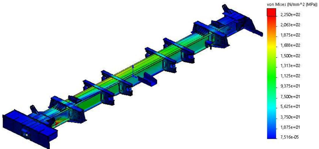
Fig. 5. The diagram of the equivalent stresses of the girder beam of the lower frame of the dump car, model 31-638, according to mode I
