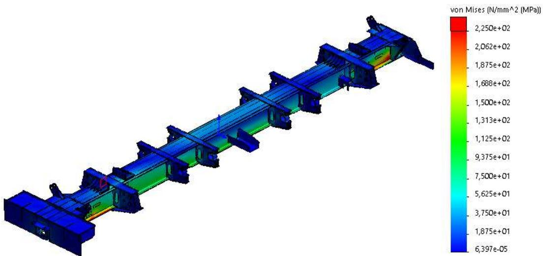
Fig. 6. The diagram of the equivalent stresses of the girder beam of the lower frame of the dump car, model 31-638, according to mode I<sub>e</sub>
