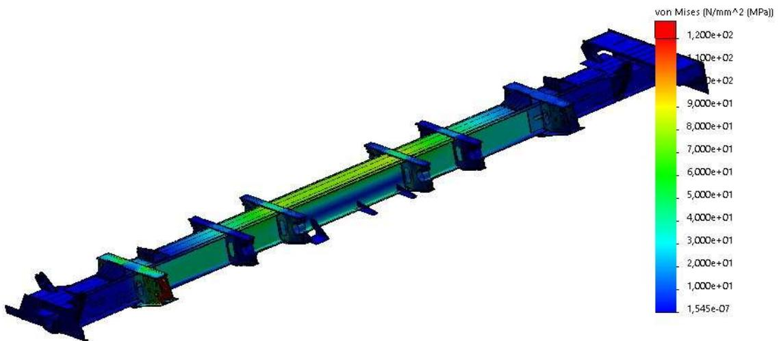
Fig. 9. The diagram of the equivalent stresses of the girder beam of the lower frame of the dump car, model 31-638, according to mode  $II_{rm2}$
