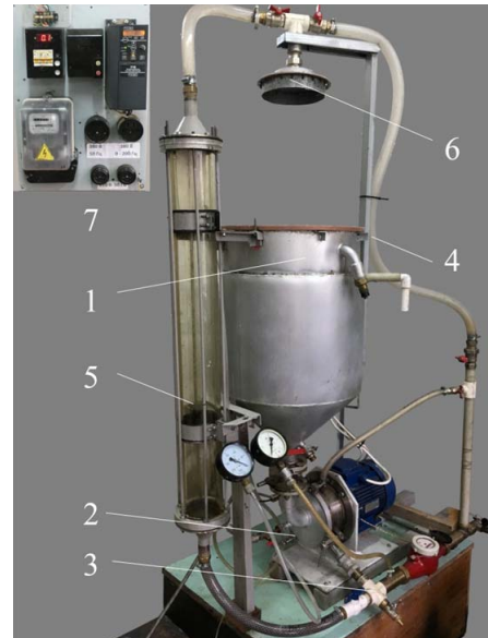
Fig. 1. Aeration and oxidation installation of the rotor type: 1 – reactor; 2 – rotary-pulsation apparatus; 3 – three-way faucet; 4 – recirculation circuit; 5 – filtration column; 6 – spray head; 7 – control unit
