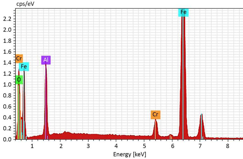
Fig. 10. Friction surface spectrum of iron aluminide coating
