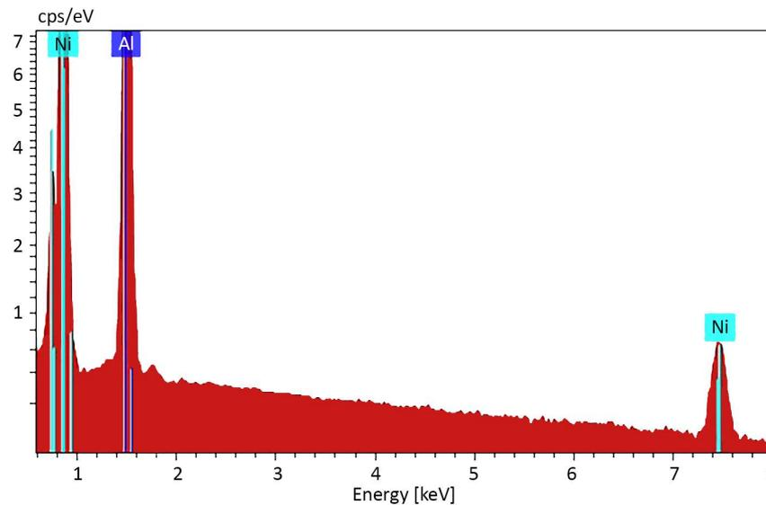
Fig. 2. The spectrum of the initial powder of aluminide nickel
