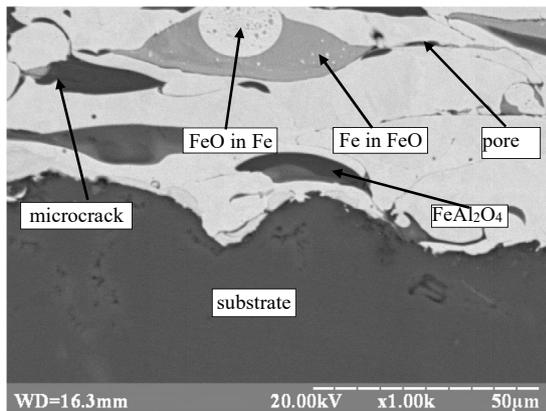
Fig. 6. Microstructure of the coating of aluminide iron obtained by APS
