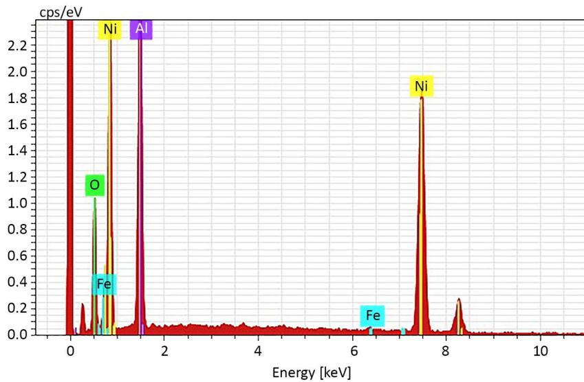
Fig. 11. Friction surface spectrum of nickel aluminide coating
