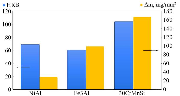
Fig. 13. Histogram of the ratio of hardness and wear of coatings made of nickel aluminide powders, iron aluminide, and 30CrMnSi steel
