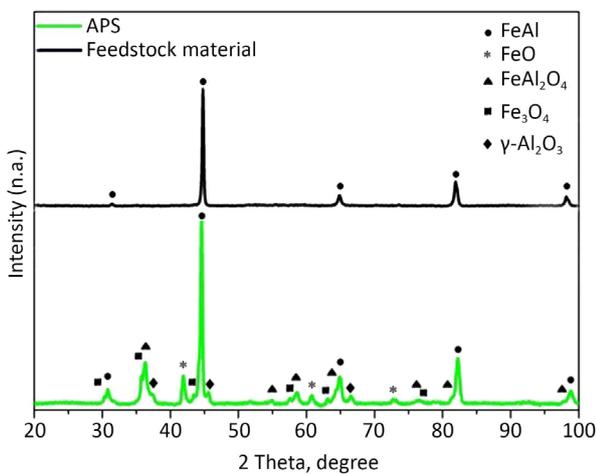
Fig. 7. XRD diffractogram of the original iron aluminide powder and coating of sprayed by APS method [22]
