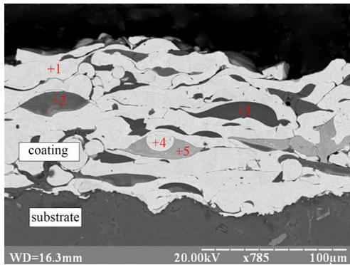
Fig. 5. The microstructure of the iron aluminide coating obtained by APS with markings to determine the chemical composition in individual areas
