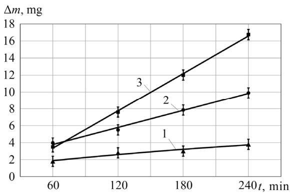
Fig. 12. Dependence of coating wear on time: 1 – from nickel aluminide powders, 2 – iron aluminide, 3 – 30CrMnSi steel
