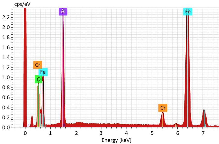
Fig. 3. APS spectrum of iron aluminide coating
