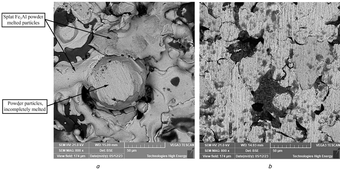
Fig. 8. Morphology of the APS surface of iron aluminide powder coating: *a* – in the original state; *b* – after friction and wear
