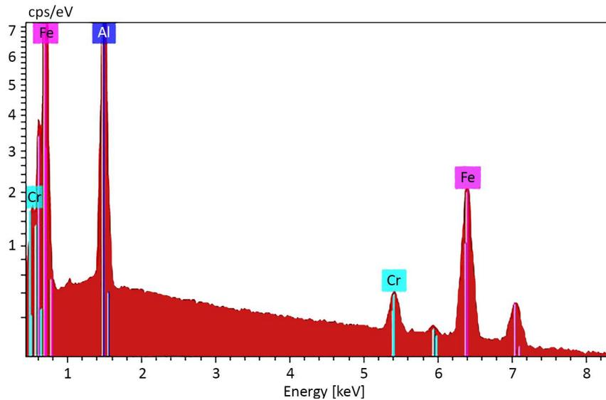
Fig. 1. Spectrum of starting iron aluminide powder
