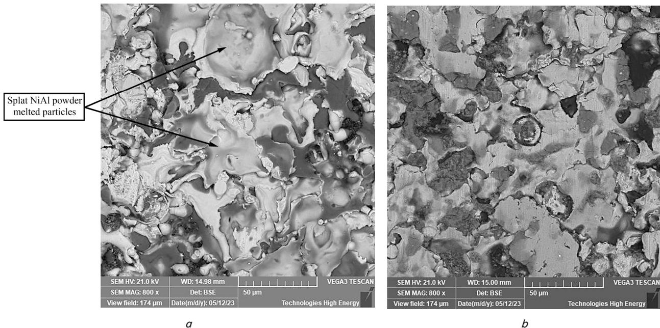
Fig. 9. Morphology of the APS surface of the nickel aluminide powder coating: *a* – in the initial state; *b* – after friction and wear
