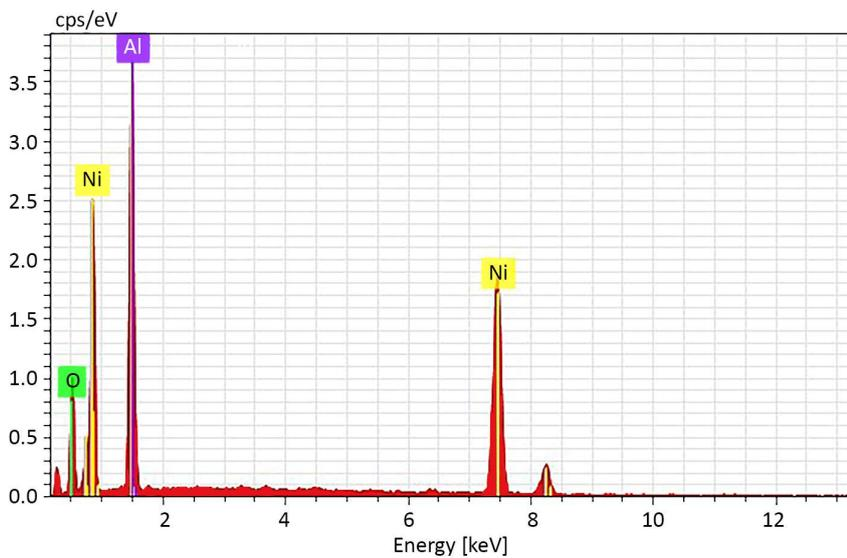
Fig. 4. APS spectrum of nickel aluminide coating
