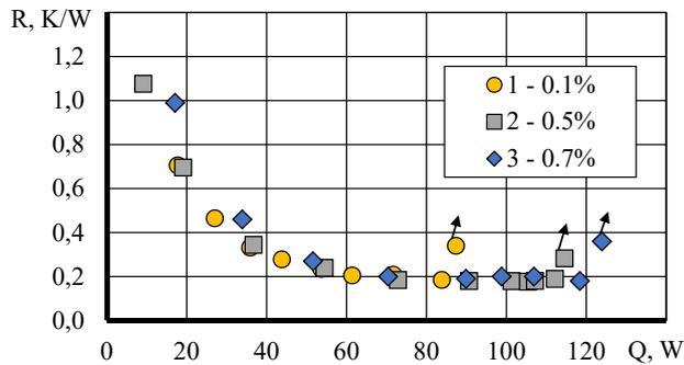
Fig. 9. Influence of nanoparticle concentration on heat transfer characteristics for  $F_r=0.59$ : 1 – 0,1 %; 2 – 0,5 %; 3 – 0,7 %
