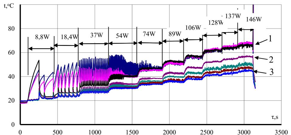
Fig. 2. Dependence of the temperature of the thermosyphon wall with an inner diameter of  $5.0 \cdot 10^{-3}$  m on time when the heat flow changes ( $F_f=0.44$ ) (water heat-carrier based on a mixture of carbon nanotubes and attapulgite (0.5 %)): 1 – heating zone; 2 – adiabatic zone; 3 – condensation zone
