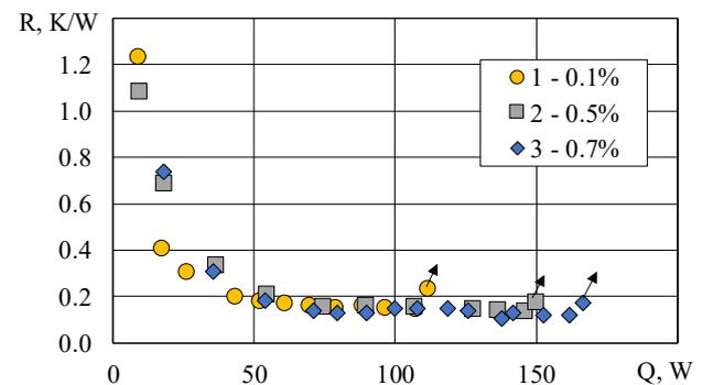
Fig. 8. Influence of nanoparticle concentration on heat transfer characteristics for  $F_r = 0.44$ : 1 – 0,1 %; 2 – 0,5 %; 3 – 0,7 %
