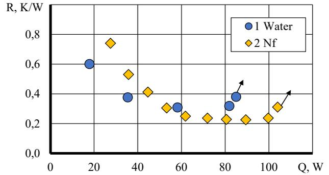
Fig. 4. Dependence of thermal resistance on the transferred heat flow for  $F_r=0.59$ : 1 – miniature thermosyphon with water; 2 – miniature thermosyphon with a water heat-carrier based on a mixture of carbon nanotubes and attapulgite (0.5 %)
