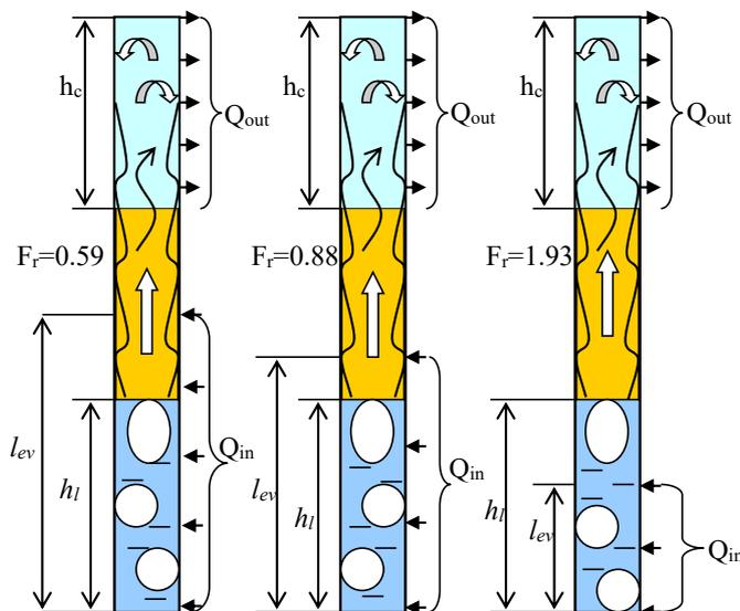
Fig. 7. Scheme of operation of a thermosyphon with an inner diameter of  $5 \cdot 10^{-3}$  m at different  $F_r$  ( $h_c = \text{const}$ )
