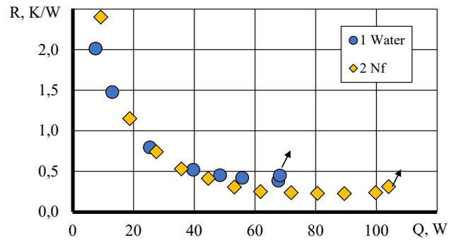
Fig. 5. Dependence of thermal resistance on the transmitted heat flow for  $F_r=0.88$ : 1 – thermosyphon with water; 2 – thermosyphon with a water heat-carrier based on a mixture of carbon nanotubes and attapulgite (0.5 %)
