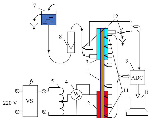
Fig. 1. Scheme of an experimental bench for the study of heat transfer characteristics of evaporative-condensing systems
