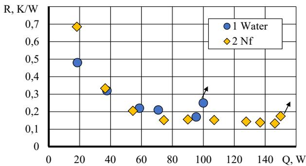
Fig. 3. Dependence of thermal resistance on the transmitted heat flow for  $F_r=0.44$ : 1 – miniature thermosyphon with water; 2 – miniature thermosyphon with a water heat-carrier based on a mixture of carbon nanotubes and attapulgite (0.5 %)
