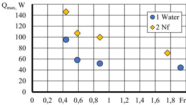
Fig. 6. Dependence of the maximum transferred heat flow on the filling factor: 1 – thermosyphon with water; 2 – thermosyphon with a water heat-carrier based on a mixture of carbon nanotubes and attapulgite (0.5 %)
