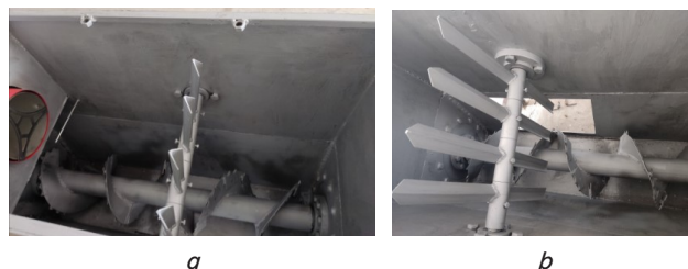
Fig. 4. General view of the working area of the grinder-mixer-dryer at idle: a – right side view; b – left view
