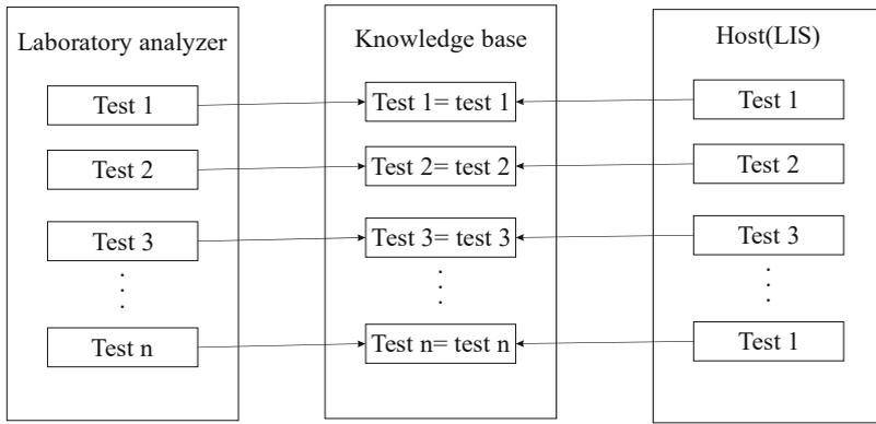
Fig. 3. Knowledge base of relationships between the analyzer and the laboratory information system
