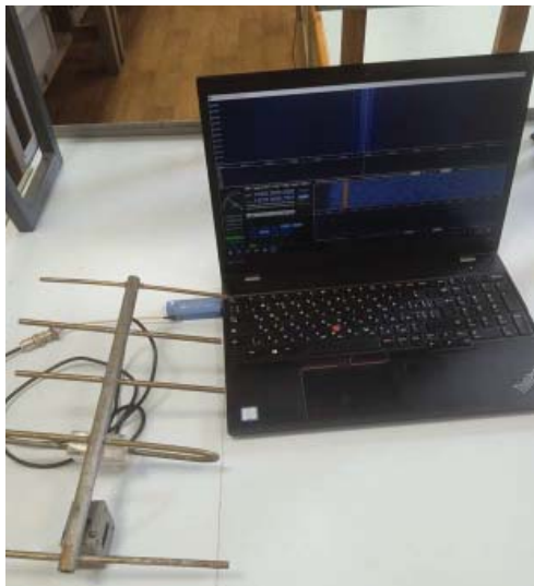
Fig. 8. Experimental installation using a directional antenna
