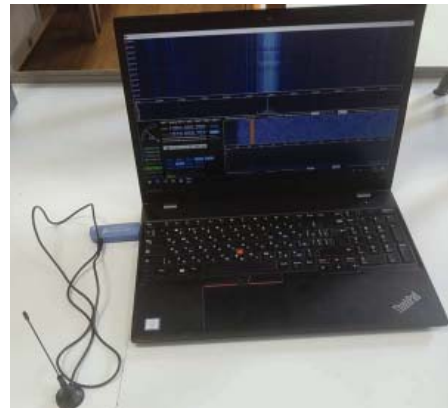
Fig. 6. Experimental installation using a non-directional antenna
