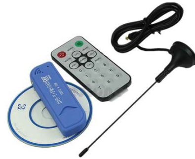
Fig. 5. Receiver DVB-T+FM+DAB 820T2 & SDR with non-directional antenna 15 cm (included)
