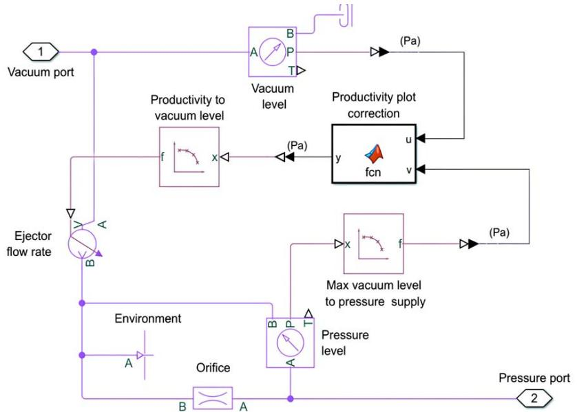
Fig. 4. Block diagram of a computer model of a mechatronic vacuum ejector
