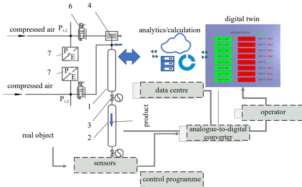
Fig. 1. Structural diagram of the hybrid mechatronic dosing and packaging module for liquid products: 1 – receiver, product feeder; 2 – portion control receiver for dose measurement; 3 – flow meter; 4 – vacuum ejector; 5 – electromagnetic pneumatic valve; 6 – pulse width modulation driver
