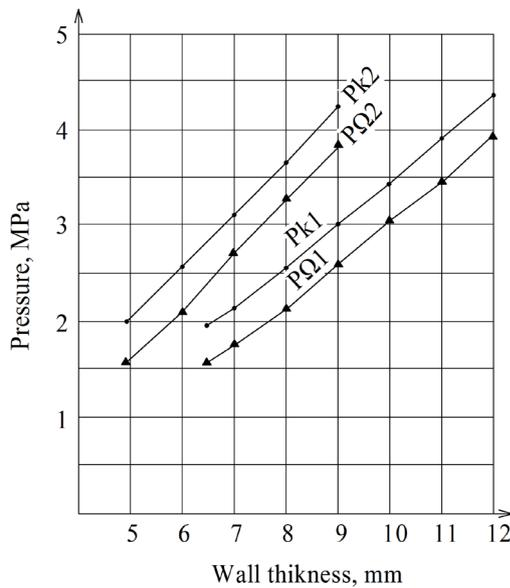
Fig. 2. Comparison of strength characteristics of pipes with a diameter of 168 mm (index 1) and 127 mm (index 2)
