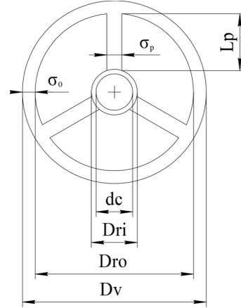
Fig. 4. Shape of the intake valve holes:  $D_v$  – diameter of the valve disc;  $D_{ro}$  – outer diameter of the annular hole;  $D_{ri}$  is its internal diameter;  $d_c$  – diameter of the vertical valve rod;  $\sigma_0$  – distance of the hole from the edge of the disk;  $\sigma_p$  – thickness of the partition;  $L_p$  – length of the partition
