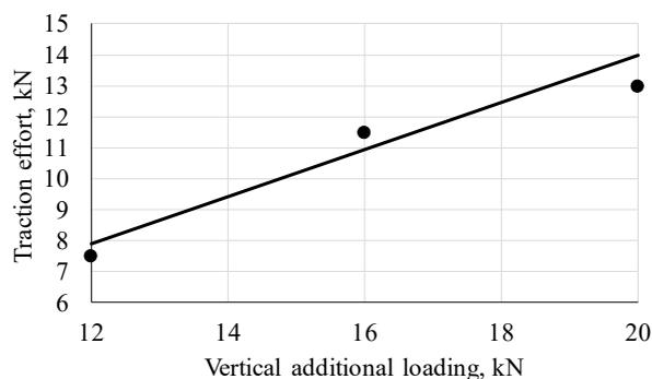
Fig. 6. Comparing the results of theoretical and experimental studies on the determination of traction resistance of the shredder roller: — — theoretical dependence; • — experimental data
