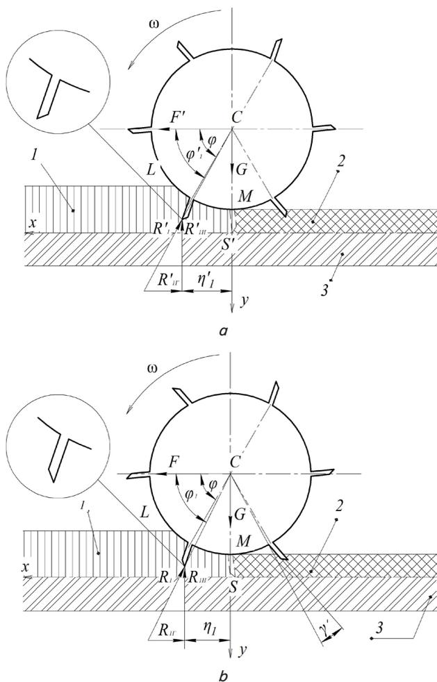
Fig. 1. The scheme of interaction of the shredder roller blade with the plant environment: 1 – plant remains; 2 – a layer of crushed plant remains; 3 – soil; a – the cutting edge of the blade coincides with the direction of rotation of the roller drum (assembly diagram 1); b – the cutting edge is installed in the direction opposite to the direction of rotation of the drum (assembly diagram 2)
