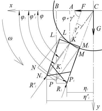
Fig. 2. Calculation scheme of superimposed images of the interaction of the blades of the shredder roller with the plant environment according to scheme 1 and scheme 2
