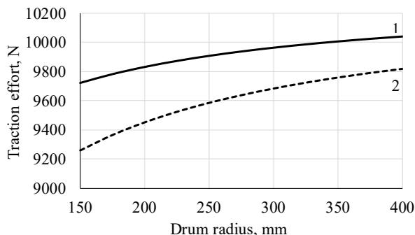
Fig. 4. Dependence of the traction force on the radius of the drum for blad: 1 – the cutting edge coincides with the direction of rotation of the roller drum (scheme 1); 2 – the cutting edge is set in the direction opposite to the direction of rotation (scheme 2) at  $a=0.3$  m/s;  $g=9.81$  m/s;  $\varphi=50^\circ$ ;  $h_t=80$  mm;  $\gamma'=12^\circ$ ;  $b=8$  mm;  $G=15000$  N
