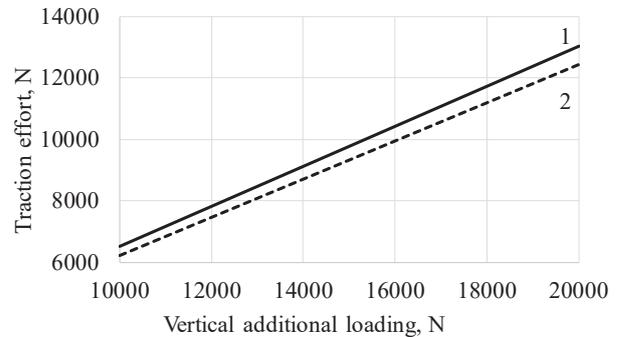
Fig. 3. Dependence of traction effort on vertical post-loading for blades: 1 – the cutting edge coincides with the direction of rotation of the roller drum (scheme 1); 2 – the cutting edge is set in the direction opposite to the direction of rotation (diagram 2) at  $\alpha=0.3 \text{ m/s}^2$ ;  $g=9.81 \text{ m/s}^2$ ;  $r_d=165 \text{ mm}$ ;  $\varphi=50^\circ$ ;  $h_t=80 \text{ mm}$ ;  $\gamma'=12^\circ$ ;  $b=8 \text{ mm}$
