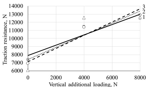
Fig. 5. Change in the traction resistance of the shredder roller depending on the vertical additional loading under conditions of movement at a speed of: 1 – 7.45 km/h; 2 – 13.6 km/h; 3 – 22.0 km/h
