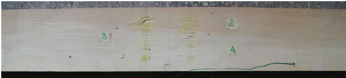
Fig. 8. Crack patterns of sample 1-Cn
