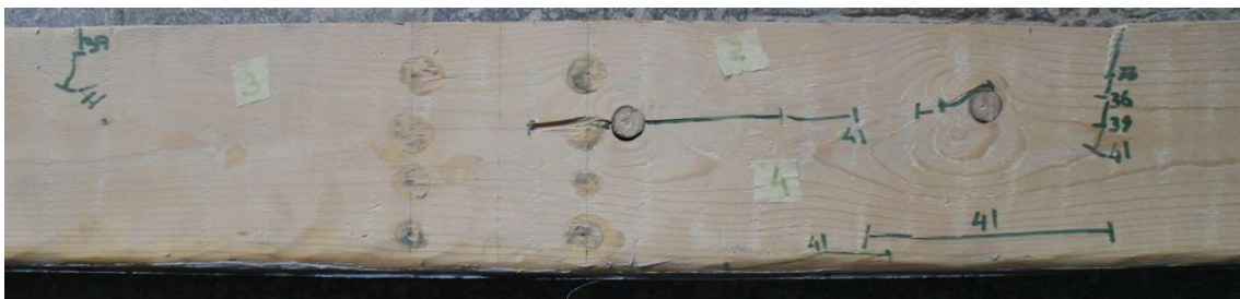
Fig. 10. Crack patterns of sample 1-PI
