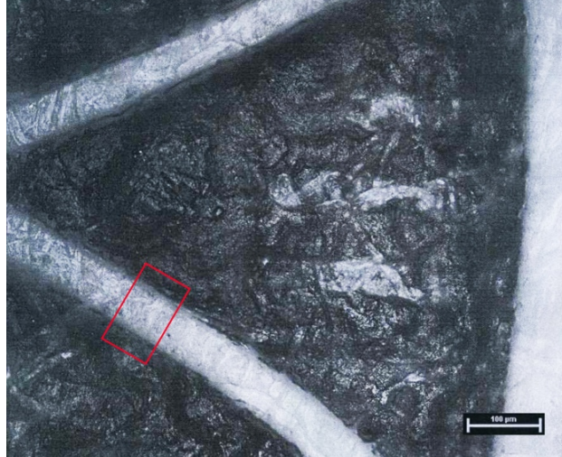
Fig. 7. Section of the mark for the visually impaired on the UAH 20 banknote, which was studied
