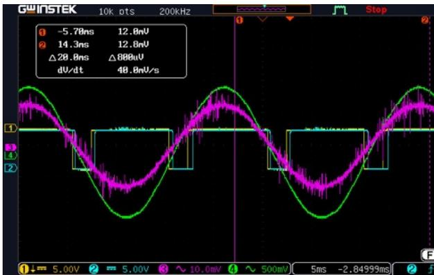
Fig. 3. Oscillogram of the reed switch, analog and discrete Hall sensors operation
