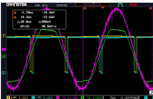
Fig. 4. Oscillogram of the reed switch, analog and discrete Hall sensor operation
