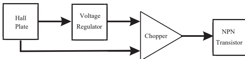
Fig. 9. Hall sensor SS443A circuit diagram
