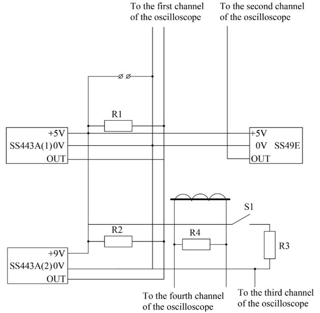
Fig. 7. Measurement scheme
