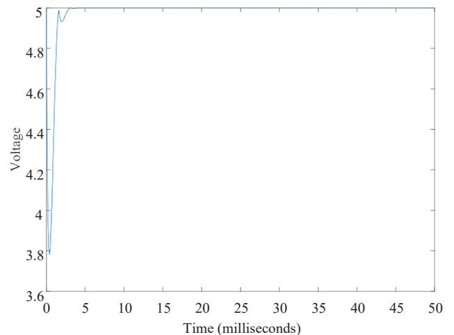
Fig. 2. Reed switch actuation behavior
