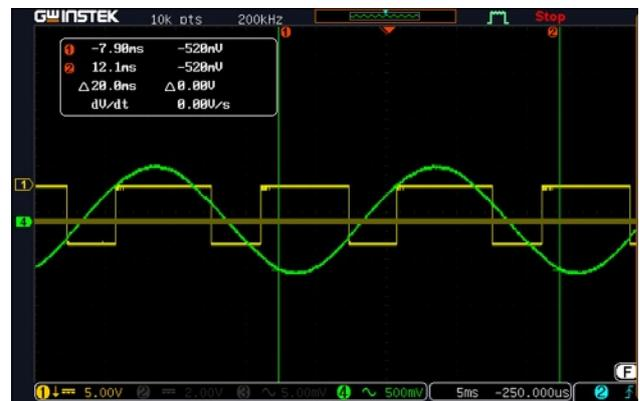
Fig. 8. Oscillogram of operation of the discrete Hall sensor under the influence of a sinusoidal signal
