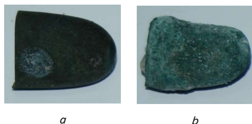
Fig. 12. Study of high-temperature salt corrosion of alloys CM93-VI and CM96-VI with boron concentration: a – 1.0 % by weight; b – 1.2 % by weight
