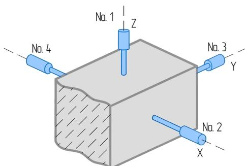
Fig. 4. Schematic diagram of testing a cement sample
