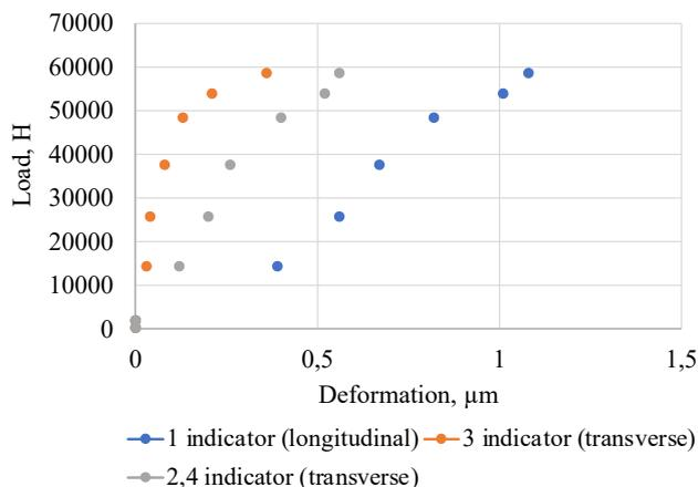
Fig. 7. Deformation of the cement stone for each indicator, 0.5 % fiber
