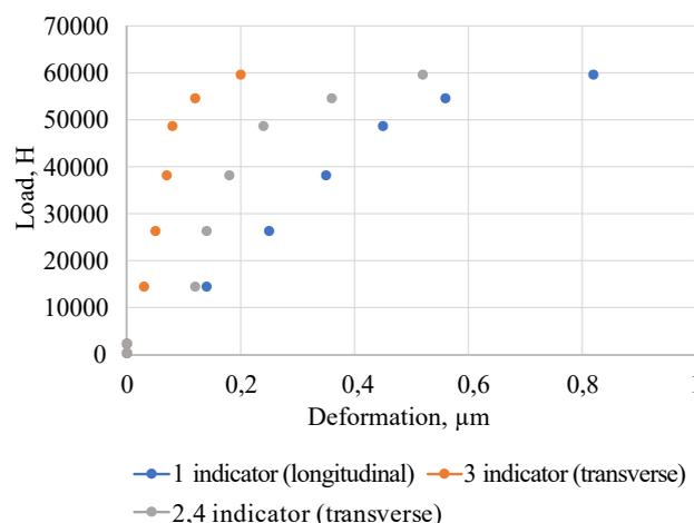
Fig. 5. Deformation of cement stone for each indicator, pure cement
