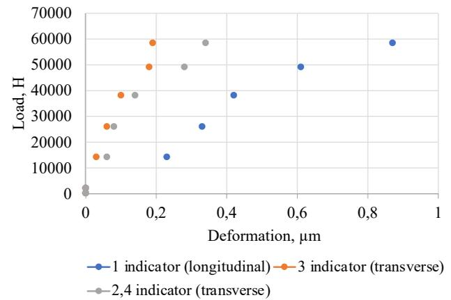
Fig. 8. Deformation of the cement stone for each indicator, 1 % fiber
