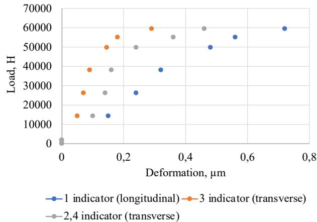
Fig. 6. Deformation of the cement stone for each indicator, 0.1 % fiber
