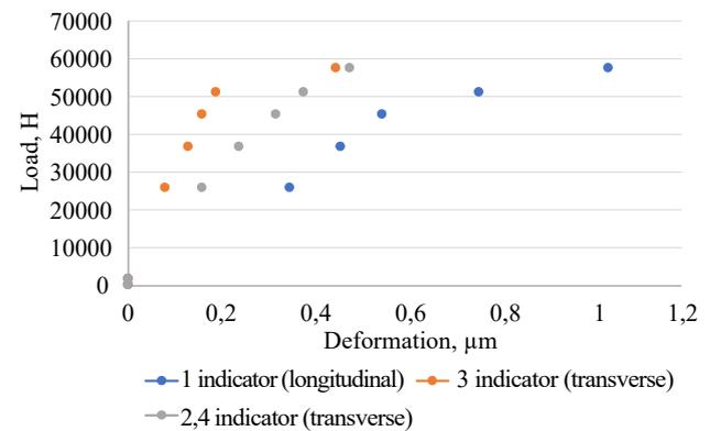
Fig. 9. Deformation of the cement stone for each indicator, 2 % fiber
