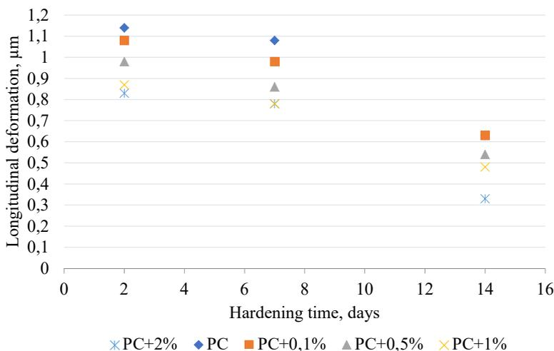
Fig. 10. Correlation of the longitudinal deformation and hardening time of the stone at various concentrations
