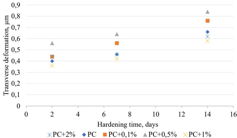
Fig. 11. Correlation of the transverse deformation according to the second and fourth indicators and hardening time of the stone at various concentrations
