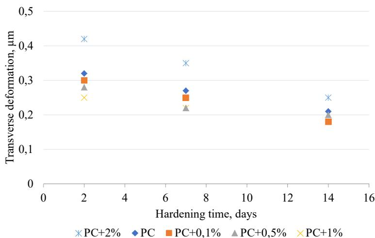
Fig. 12. Correlation of the transverse deformation according to the third indicator and hardening time of the stone at various concentrations
