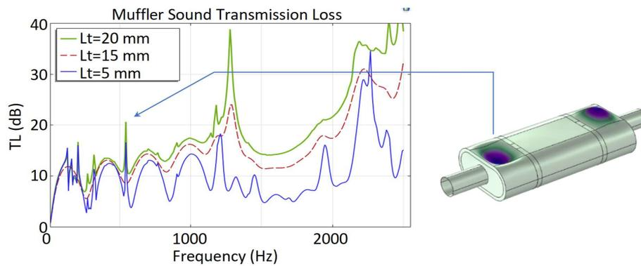
Fig. 7. Sound transmission loss of a muffler with varied shell thickness ( $Lt$ )
