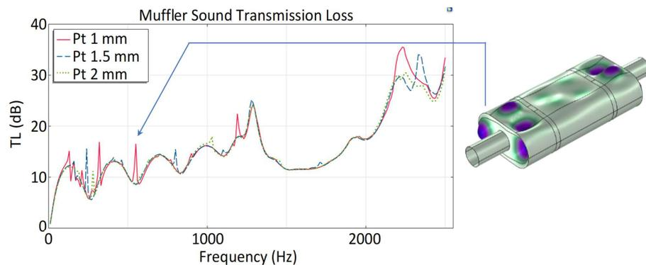
Fig. 8. Sound transmission loss of a muffler with varied shell plate thickness ( $Pt$ )
