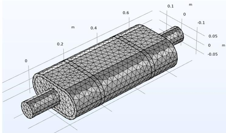
Fig. 3. Meshed geometry of an exhaust muffler with shell
