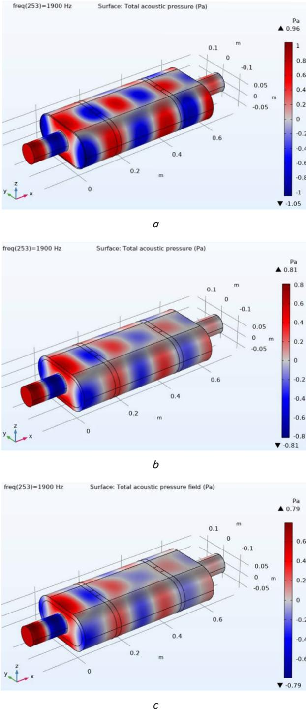
Fig. 5. Total acoustic pressure of a muffler with shell for varied shell thickness: *a* –  $Lt=5$  mm; *b* –  $Lt=15$  mm; *c* –  $Lt=20$  mm
