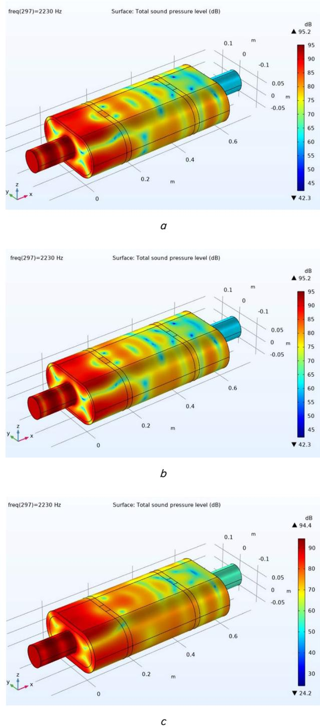
Fig. 6. Sound Pressure level of a muffler with shell for varied shell thickness: *a* –  $Lt=5$  mm, *b* –  $Lt=15$  mm, *c* –  $Lt=20$  mm
