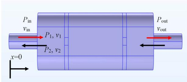
Fig. 1. Schematic diagram of the proposed shelled muffler
