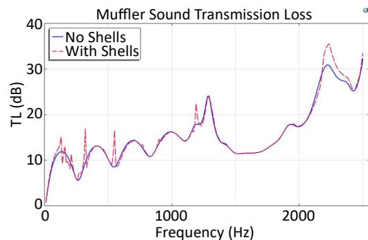
Fig. 4. A comparison of two cases of mufflers, with no shells and with shells
