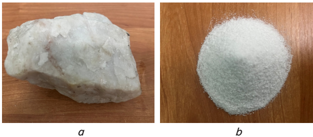
Fig. 1. Quartzite samples: a – quartz ore d=70.3 mm; b – crushed quartzite d=0.1\div 0.4 mm
