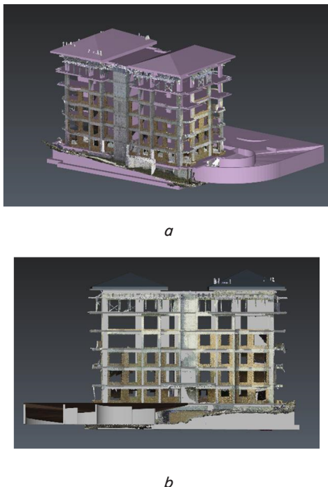
Fig. 7. Overlapping BIM model with laser scan model; a – front view; b – axonometric perspective (prepared by authors)
