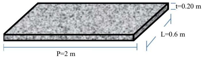
Fig. 1. Dimensions of f_c 30 MPa concrete slab specimens
