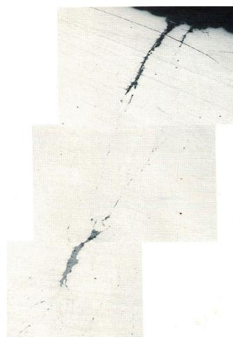
Fig. 5. Microstructure of axial defects of spherical bottom after roughing (x50)
