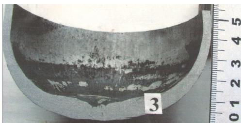
Fig. 3. Macro-sections of bottom after roughing
