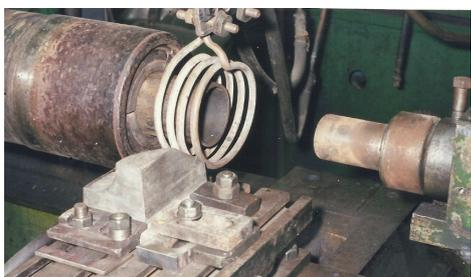
Fig. 2. Induction heating of a pipe blank before roughing
