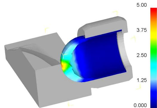
Fig. 1. Finite element model of the process of tangential roughing with a friction tool at the final stage
