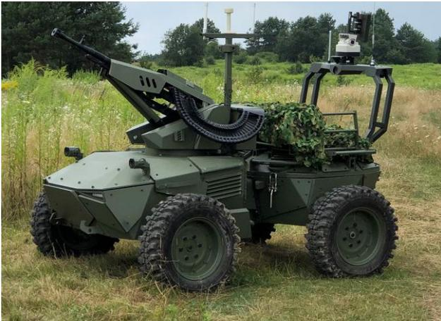
Fig. 1. Ukrainian ground robotic system «Ironclad» from Roboneers
