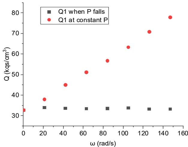
Fig. 4. Flow curves of the installation fluid with a pre-pressure of 0.25 kgf/cm<sup>2</sup> through throttle holes with a diameter of 3 mm
