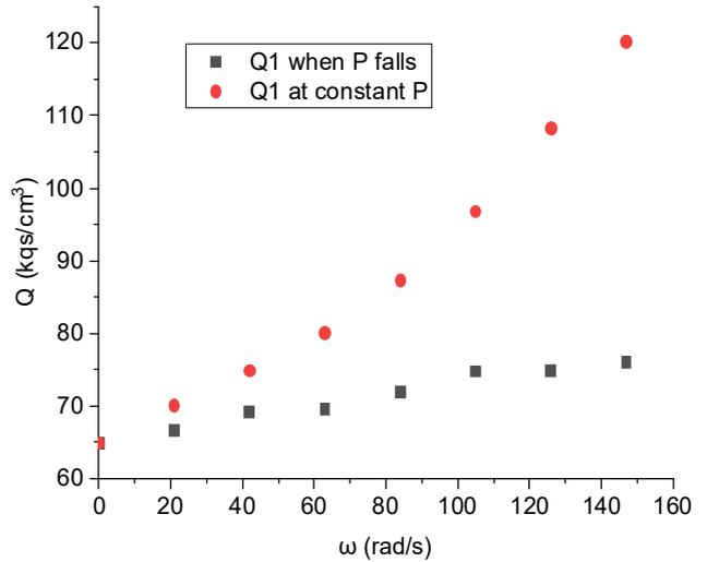
Fig. 6. Flow curves of the installation fluid with a pre-pressure of 1.0 kgf/cm<sup>2</sup> through throttle holes with a diameter of 3 mm
