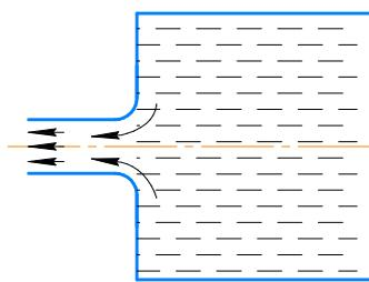
Fig. 1. Liquid flow through throttle orifices: the outflow of liquid from the cylindrical nozzle
