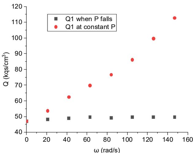
Fig. 5. Flow curves of the installation fluid with a pre-pressure of 0.5 kgf/cm<sup>2</sup> through throttle holes with a diameter of 3 mm
