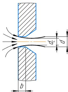
Fig. 2. Liquid flow through throttle orifices: the outflow of liquid through the opening of a thin wall
