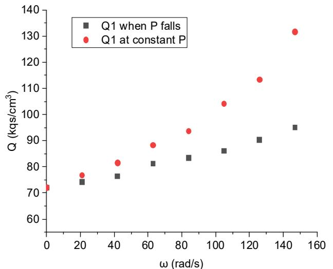
Fig. 7. Flow curves of the installation fluid with a preliminary pressure of 1.5 kgf/cm<sup>2</sup> through throttle holes with a diameter of 3 mm
