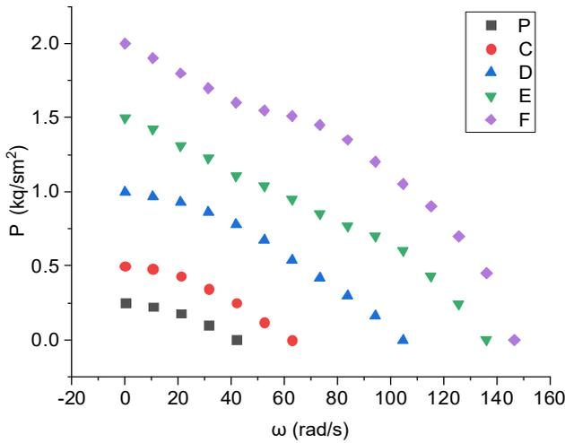
Fig. 3. Pressure drop curves with increasing rotor angular velocity
