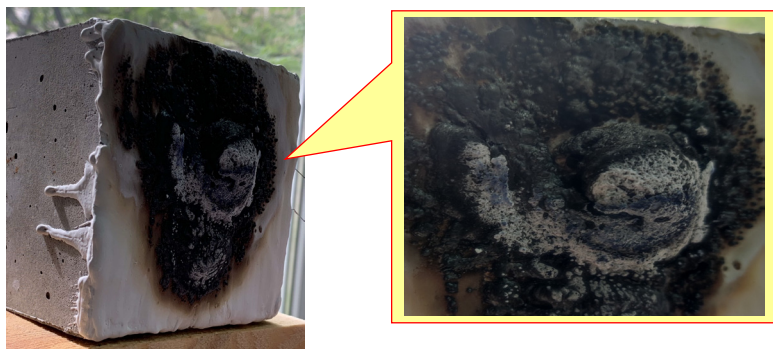
Fig. 5. Foam coke layer formation
