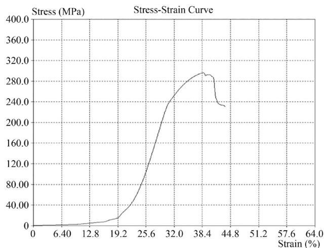
Fig. 2. Graph of the relationship between tensile strength and strain of combined directional welded joints (longitudinal+transverse) with a current strength of 100 A
