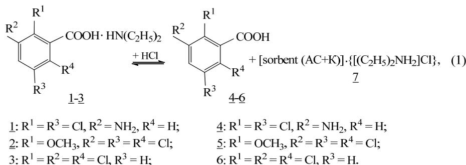
Fig. 1. General scheme for the extraction of chemicals from unusable pesticides of the general formula R<sup>1</sup>R<sup>2</sup>R<sup>3</sup>R<sup>4</sup>C<sub>6</sub>HCOOH·HN(C<sub>2</sub>H<sub>5</sub>)<sub>2</sub>
