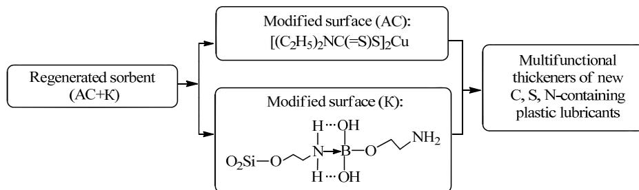
Fig. 3. Scheme of formation of structural framework fragments of new C, S, N-containing plastic lubricants
