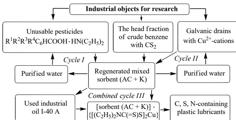
Fig. 2. Basic technological scheme for obtaining C, S, N-containing plastic lubricants using industrial waste from various industries
