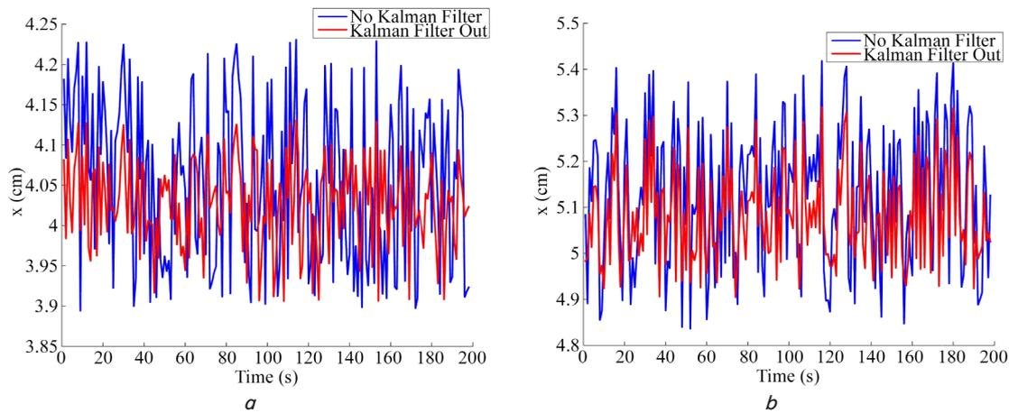
Fig. 7. Graph of Kalman’s filtering results against reference distance: *a* – reference distance 4.0 cm; *b* – reference distance 5.0 cm
