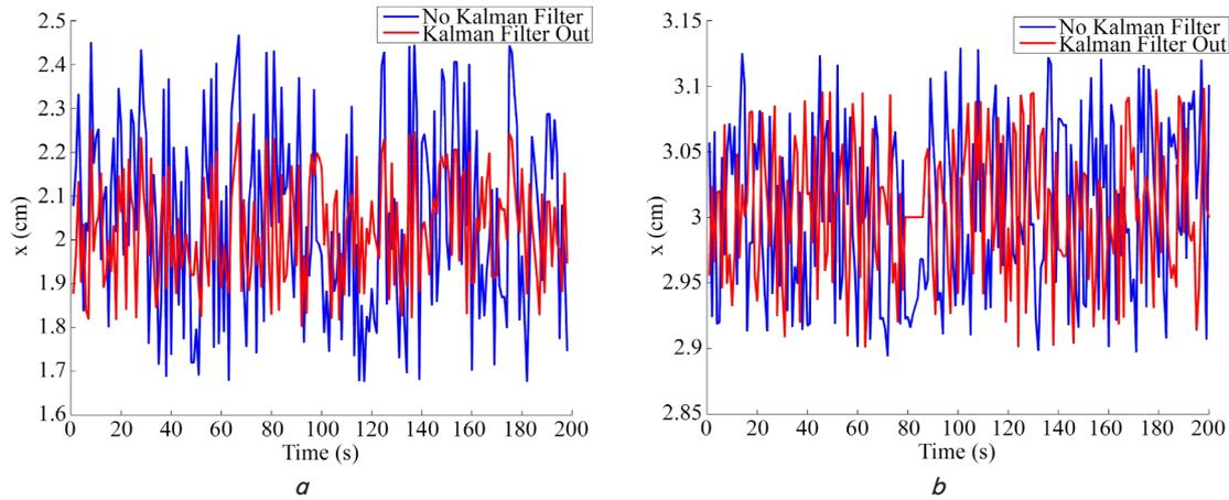
Fig. 6. Graph of Kalman’s filtering results against reference distance: *a* – reference distance 2.0 cm; *b* – reference distance 3.0 cm
