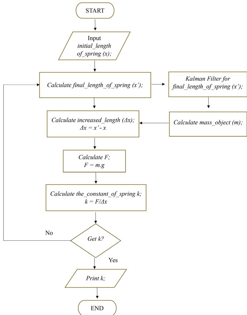
Fig. 2. Flowchart of Hooke's law prop system with Kalman filter algorithm
