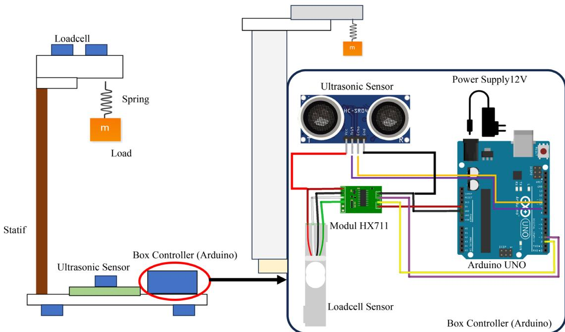
Fig. 3. Hooke's law demonstration system design uses ultrasonic sensors for distance parameter measurement
