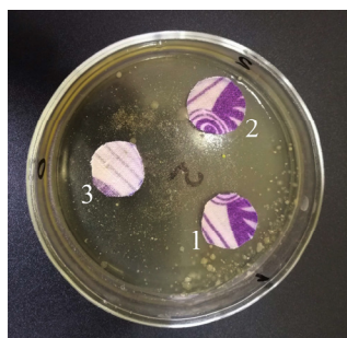
Fig. 4. The influence of synthesized ZnO nanoparticles on the development of bacterial contamination of air microflora of cotton fabric samples: 1 – without treatment; 2 – treated with synthesized nano-ZnO; 3 – processed after 5 washing cycles
