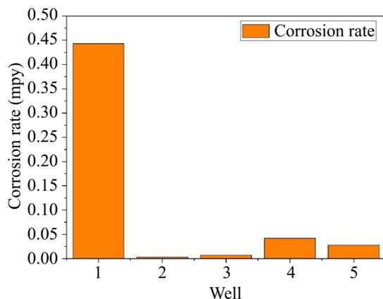
Fig. 5. The corrosion rate monitoring of the well
