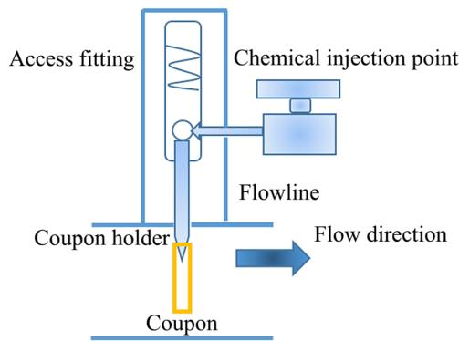
Fig. 2. The schematic illustration of the injection point to sample the fluid
