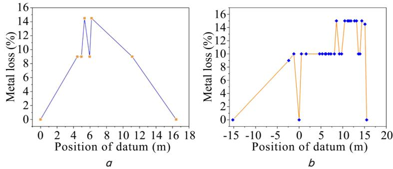
Fig. 4. The result of Ultrasonic in the form of metal loss: *a* – 18-inch; *b* – 12-inch trunklines
