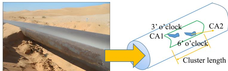
Fig. 3. The visual inspection of the 8-inch flowlines
