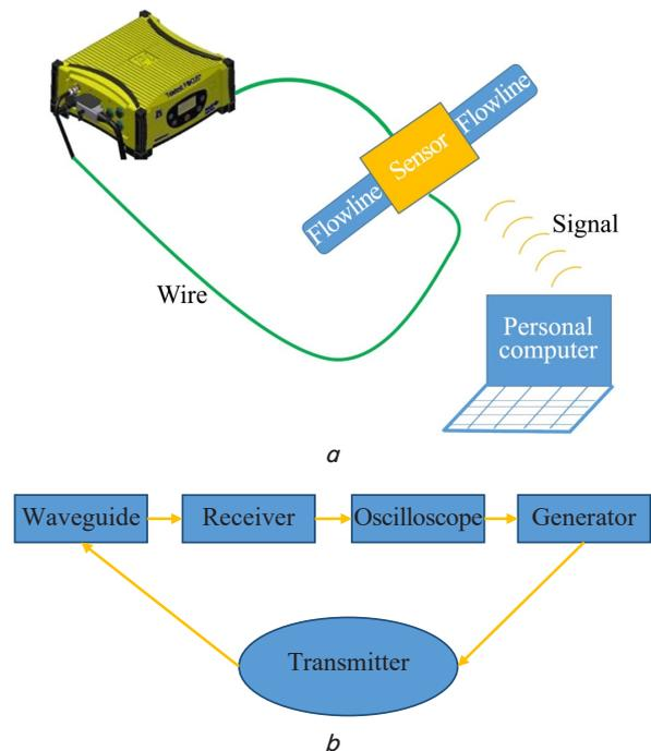
Fig. 1. The schematic illustration of: *a* – instrument and experimental ultrasonic guided wave instrument; *b* – ultrasonic operation system
