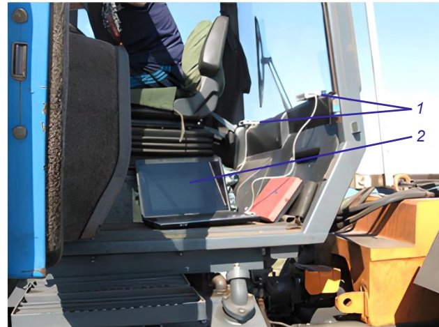
Fig. 1. Arrangement of the measuring and registration module in the tractor cab: 1 – acceleration sensors; 2 – a personal computer for data collection and archiving
