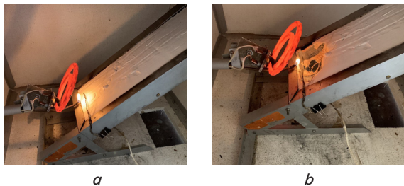
Fig. 2. Results of studying the ignition process and the spread of flame on a fire-resistant OSB-3 sample: a – the effect of the flame on the sample; b – swelling of the coating; c – a protective layer of pinocoke
