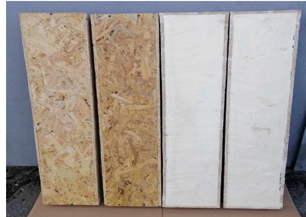
Fig. 1. The appearance of SIP-panel samples, during the application of “FIREWALL-WOOD” fire retardant on the surface of the OSB plate
