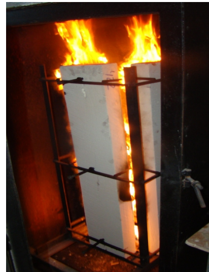
Fig. 4. Samples of sip panels during flammability tests
