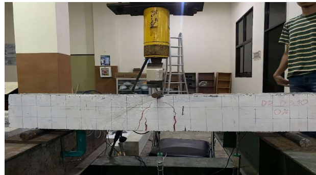
Fig. 6. Flexural collapse of polypropylene fiberized high-strength beams from medical mask waste
