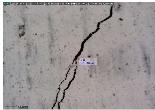
Fig. 7. Example of the results of observing crack width with a digital microscope: a – crack width at 2 kN load; b – crack width at 6 kN load
