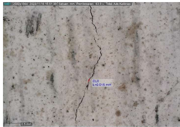
Fig. 6. Flexural collapse of polypropylene fiberized high-strength beams from medical mask waste
