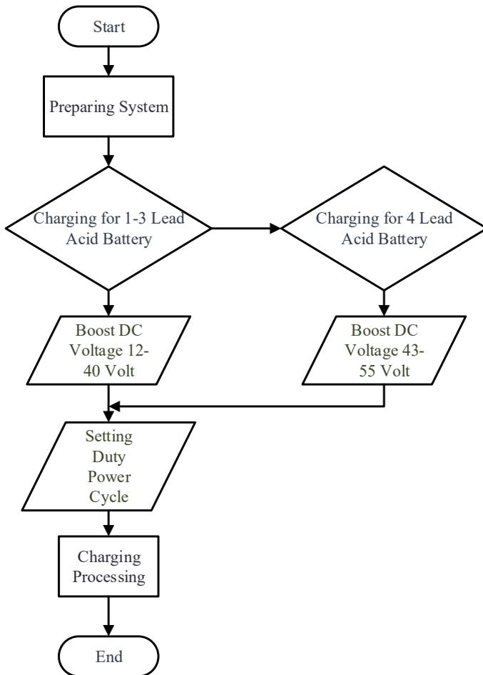
Fig. 3. Flow diagram of how smart charging works
