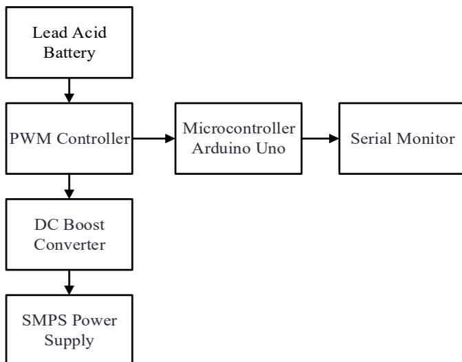
Fig. 4. Block diagram of the data retrieval process when charging
