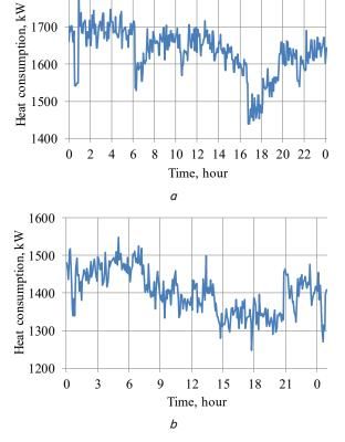
Fig. 8. Change in heating capacity: a – working day; b – day off
