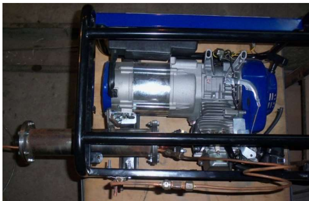
Fig. 2. Four-stroke engine 1Ch 6.8/5.4 with thermochemical conversion reactor
