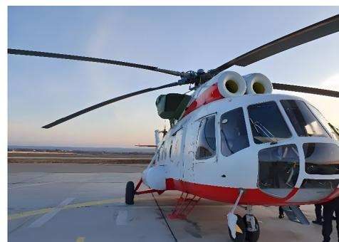
Fig. 2. Screen-exhaust device installed on the Mi-8 helicopter for experimental tests
